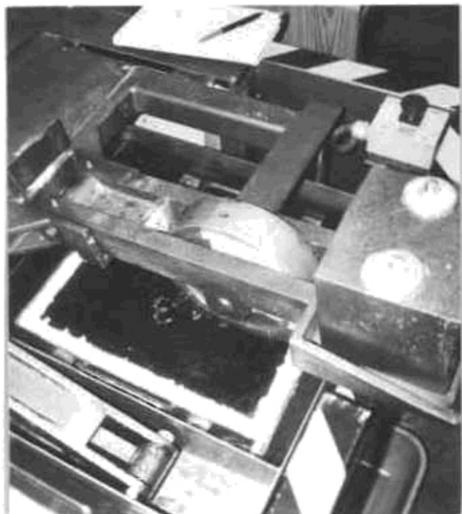
Fig. 7. A Close-up of the Hamburg Wheel-Tracking Device.
