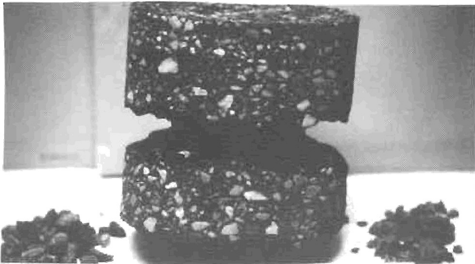
Fig. 2. The Surface of a Pavement Requiring "Complete Rehabilitation" in 12 Months.
