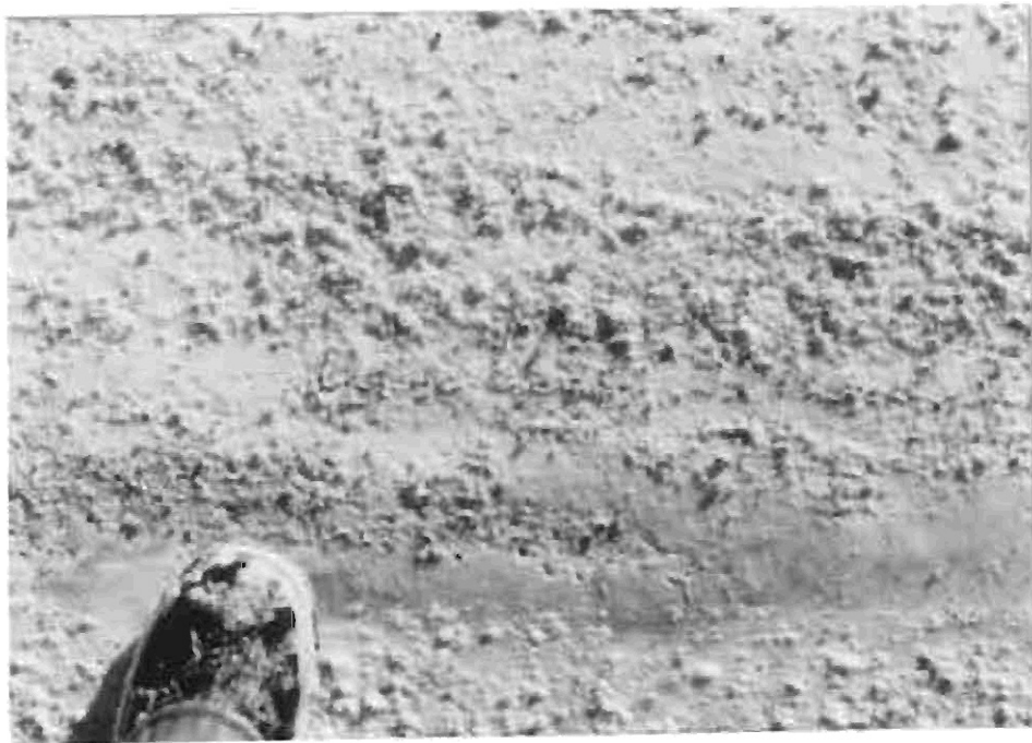
Photograph 4. Test Section 4. 5% Magnesium Chloride, 5% Salt + Sand 125 lbs. on Test Section Sunday, January 20, 1991 9:30 A.M.
