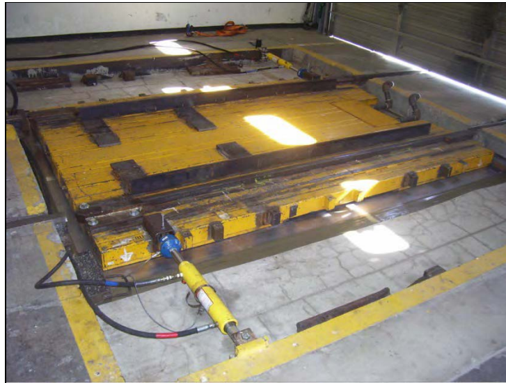
Figure 34. Photo of Truck Resistive Torque Test Setup
