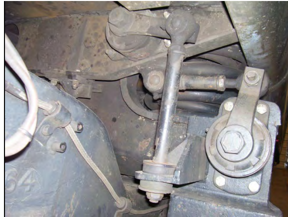
Figure 28. Vertical and Lateral Secondary Suspension Dampers on T-16 Car
