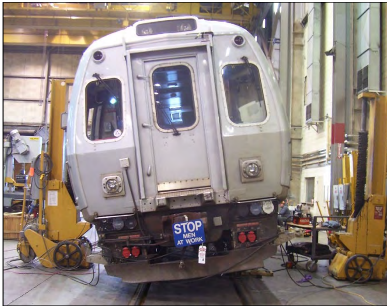
Figure 41. Lean Test Setup
