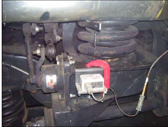
Figure 3. Secondary Suspension String Potentiometer – Vertical Displacement Measurement
