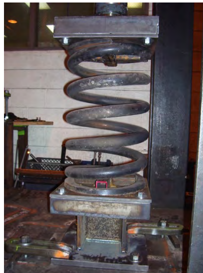
Figure 22. Suspension Spring in Load Frame
