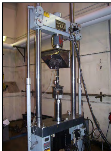
Figure 27. Damper Characterization Test
