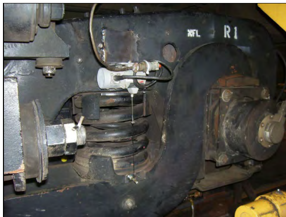
Figure 4. Primary Suspension String Potentiometer – Vertical Displacement Measurement
