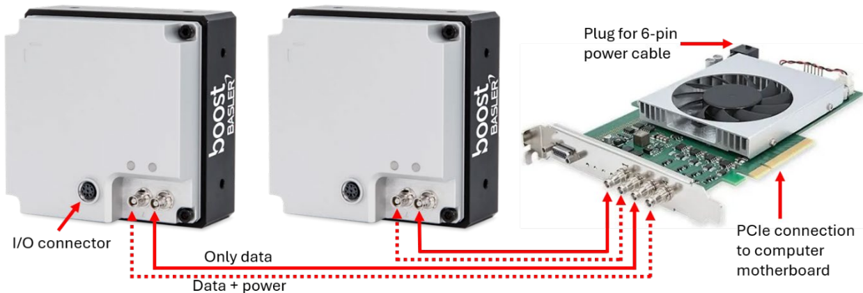
Figure 29. Illustration. Camera and interface card connections.
