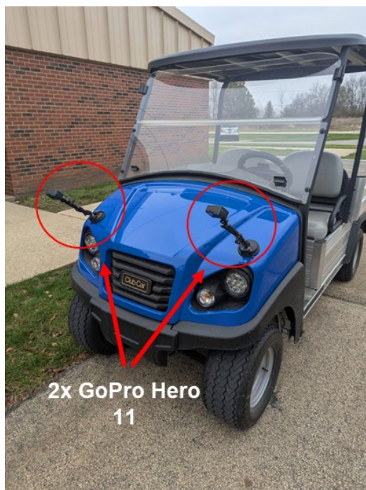
Figure 12. Photo. GoPro cameras attached to a golfcart.
