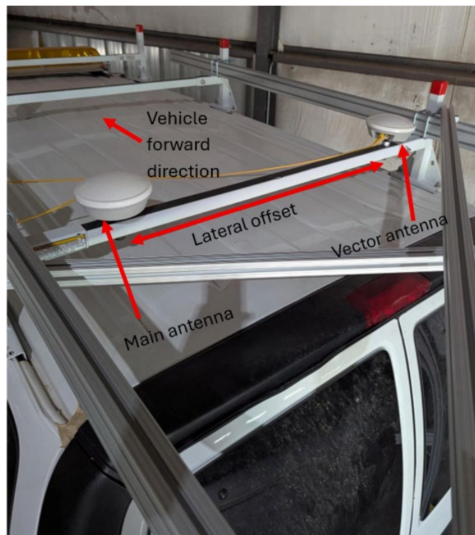
Figure 27. Illustration. Rover antenna mounting on vehicle.
