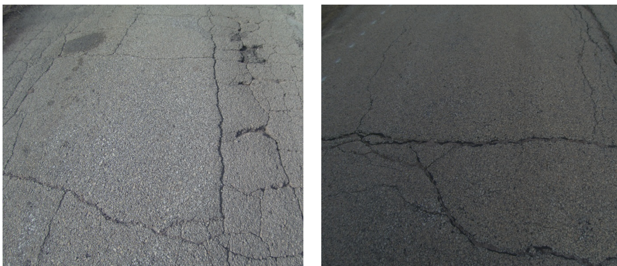
Figure 30. Photo. Effect of light intensity on image brightness.
