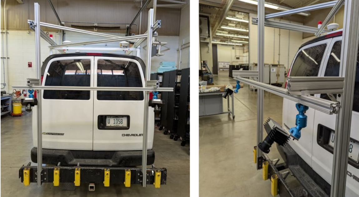
Figure 26. Photo. Camera mounting setup on a vehicle.
