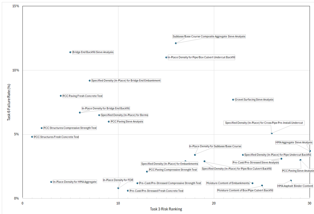
Figure 17: Risk ranking and failure rate for top 30 material testing activities
