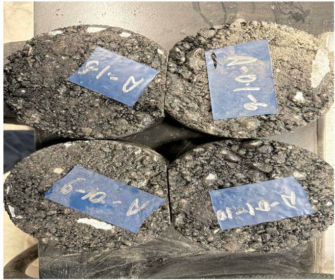
Figure 10. HWT Specimen With Perpendicular Cut
