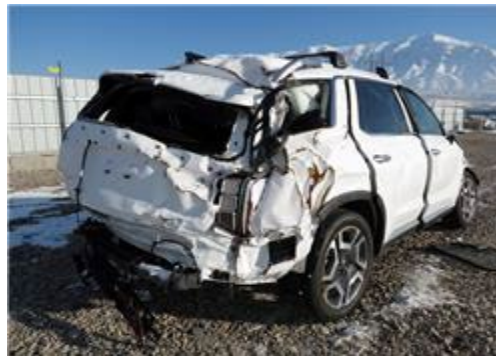
Figure 4. Greenhouse crush damage 2023 Hyundai Palisade
