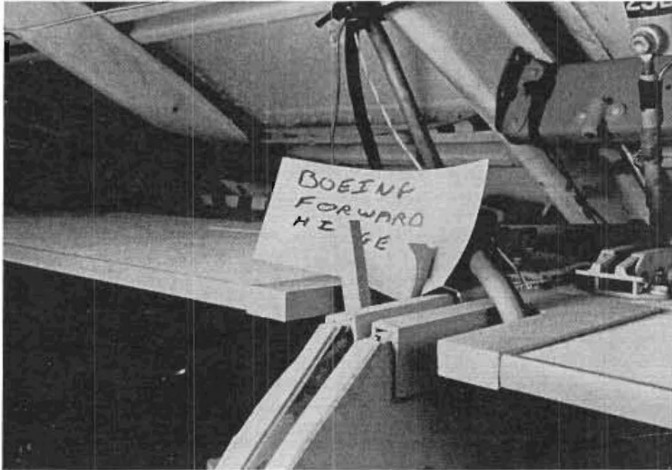
FIGURE 43. BOEING BIN BROKEN FORWARD HINGE, POSTTEST
