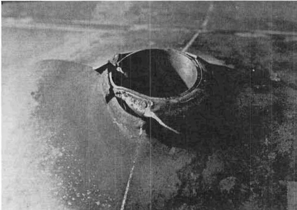
FIGURE 59. AUXILIARY FUEL TANK DRAINAGE HOLE CLOSE UP, POSTTEST
