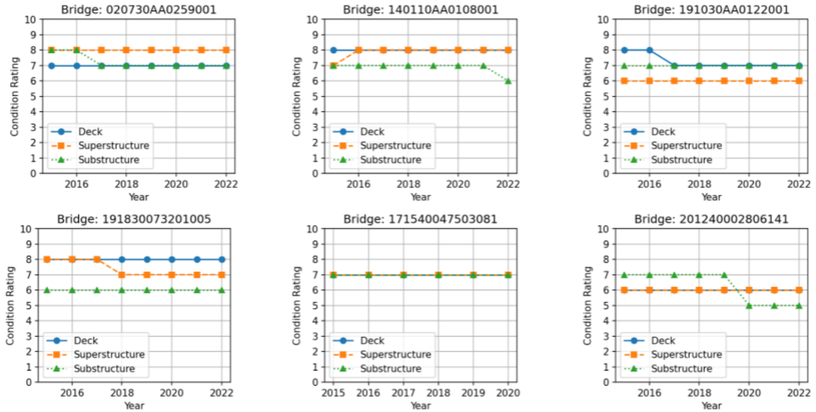
Fig. 3.2.1: Sample trends of bridge component condition ratings (2015–2022)
