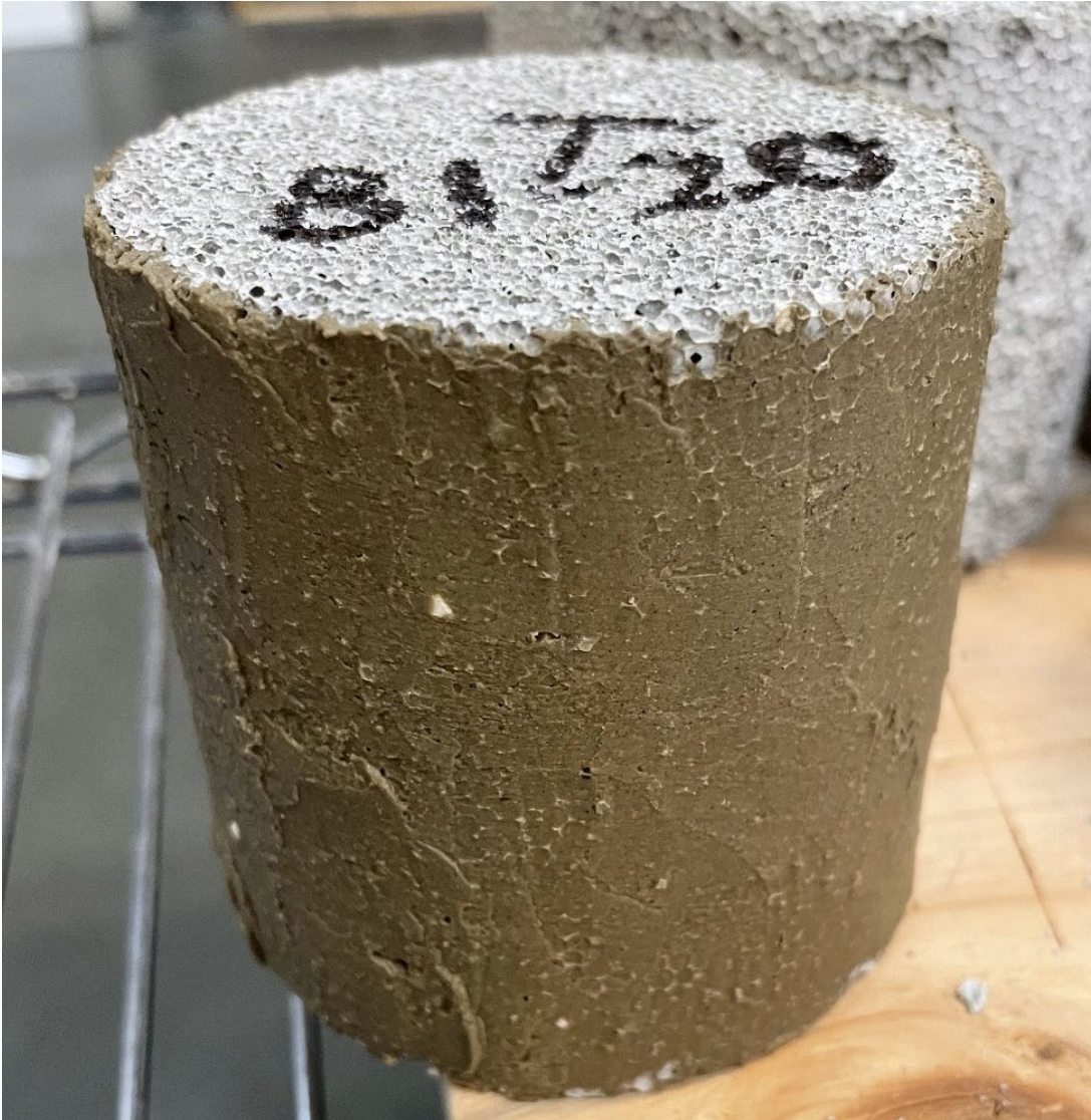
Figure 8-1 Photo of the LCC specimen with the bentonite gel sidewall treatment
