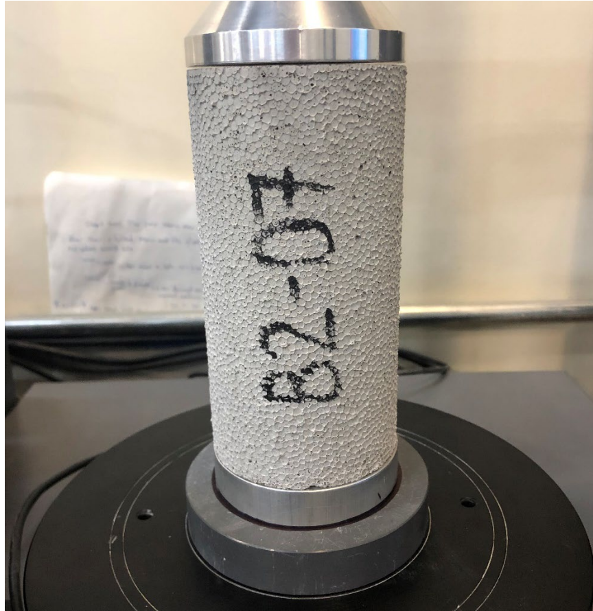
Figure 10-2 Photo of a specimen prepared for UCS testing in the load frame without padded end caps
