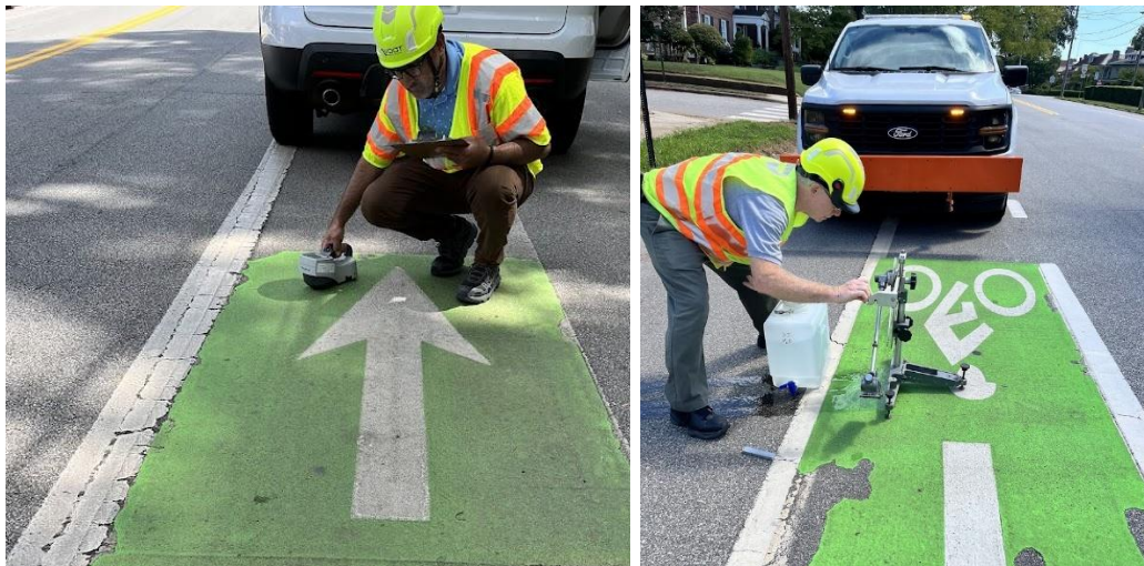
Figure 9. Collection of Green-Colored Pavement Marking Color Readings Using a Colorimeter (left) and Skid Resistance Data Using the British Pendulum Tester (right)
