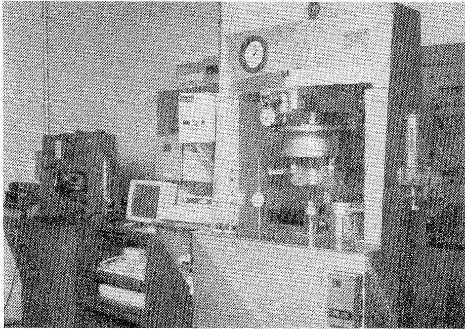
Figure 14. WES Model 4C and 8A/6B/4C Gyratory Testing Machines
