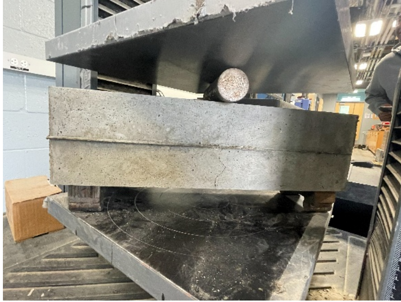
Figure 65. Image. 6 × 6 × 21 in. beam split during 3-point bending test.
