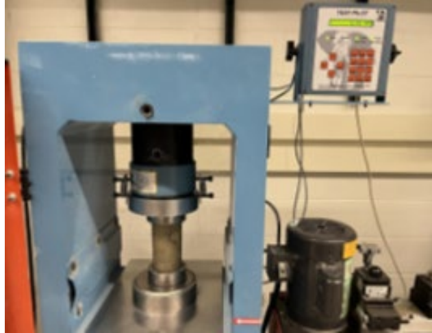
Figure 19. Image. Compression testing setup.
