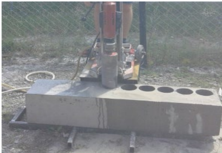
Figure 7. Image. Drilled core testing on site.
