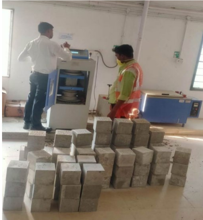
Figure 22. Image. Compressive-strength testing on concrete cubes.
