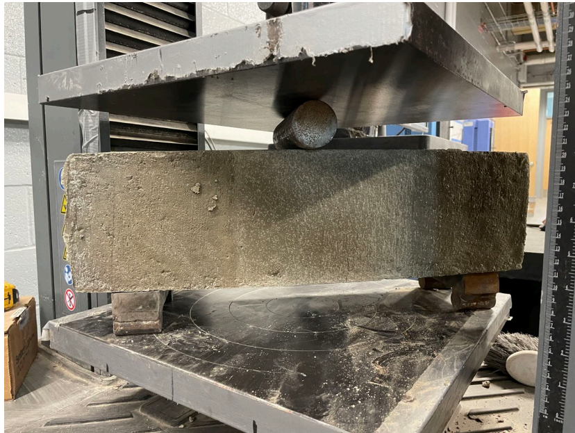
Figure 14. Image. Concrete beam flexural test in the laboratory.
