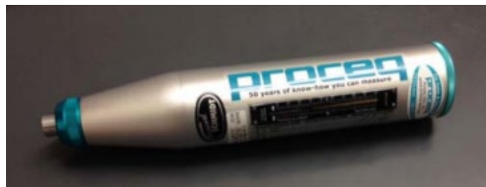
Figure 9. Image. Rebound hammer testing.
