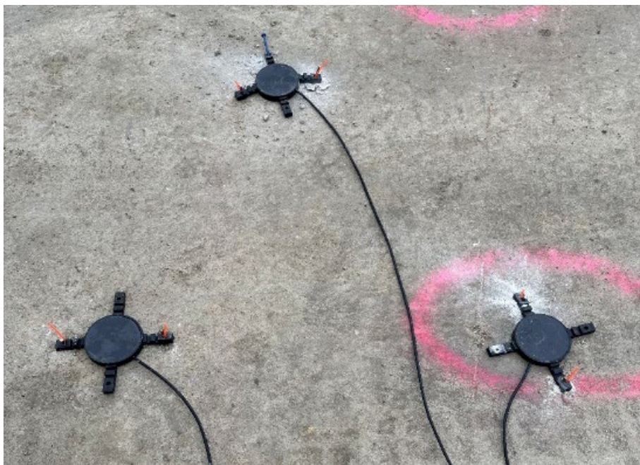
Figure 42. Photo. Sensors nailed in place.
