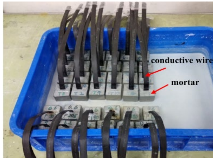
Figure 3. Image. Mortar specimens with embedded piezoelectric sensors cured in water.
