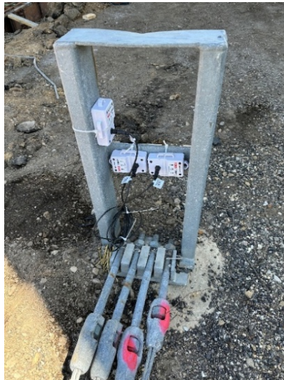
Figure 58. Image. Data loggers zip-tied to high-tension barrier terminal.
