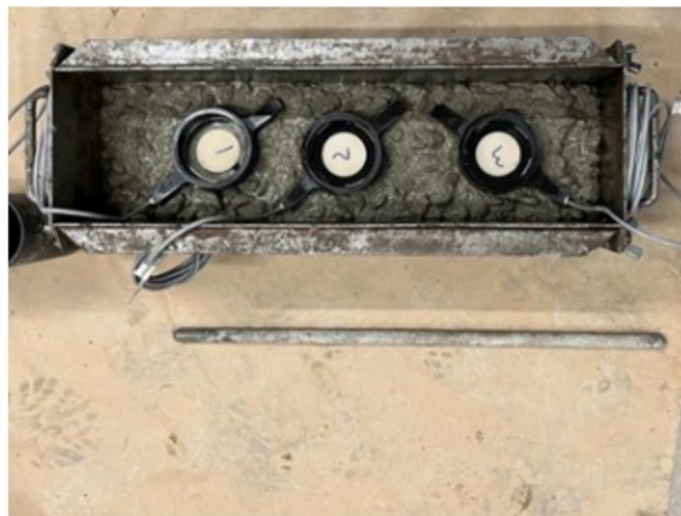
Figure 4. Image. Embedded sensors for a concrete beam.
