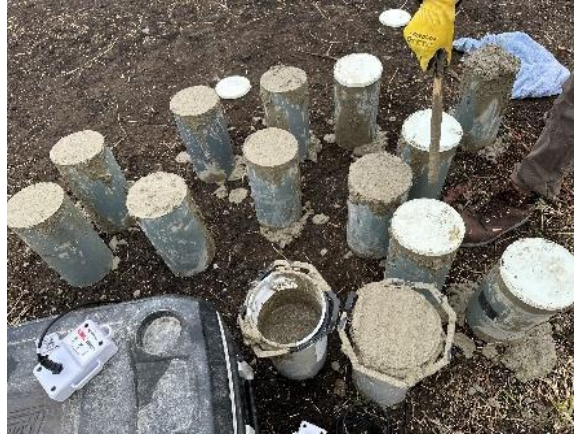
Figure 17. Image. Cylinders cast at site.
