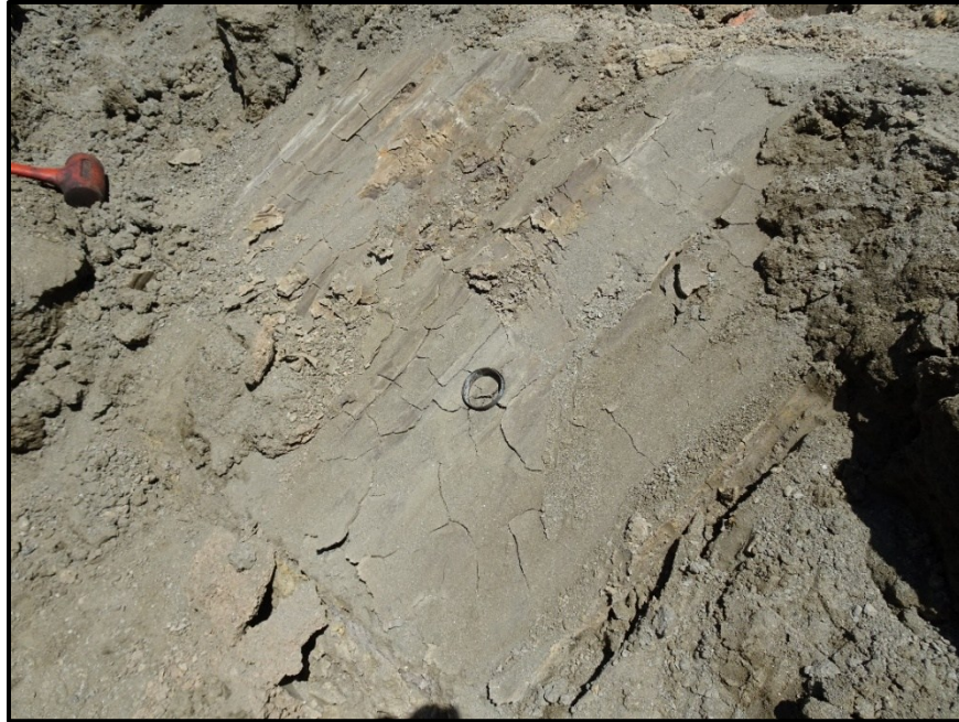
Figure 25. US 36 MP 50.05 Location of Slickensides denoting Failure Plane in Excavation with California Sampler Hand Driven to collect sample for Direct Shear.
