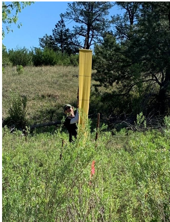
Figure 8. Using a 3-m tall vertical cover board to estimate vertical vegetation density.
