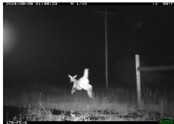
Figure 48. White-tailed deer jumping over the Geocell fence end treatment.
