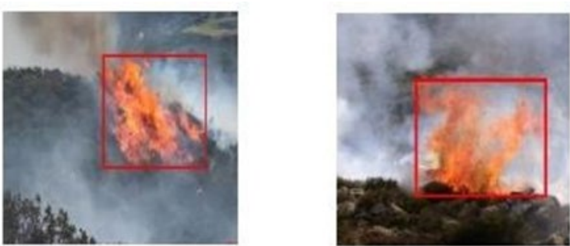
Figure 12: Fire detection using object detection showing detected region of interest
