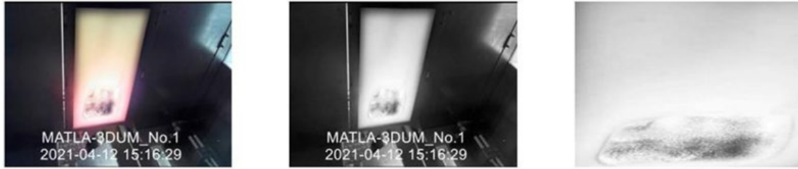
Figure 35: Charring area extraction from end-of-test frames
