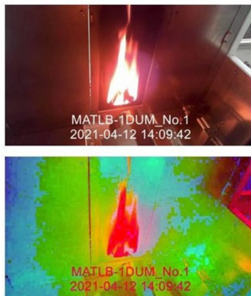
Figure 34: Flame intensity extraction by converting images to HSV
