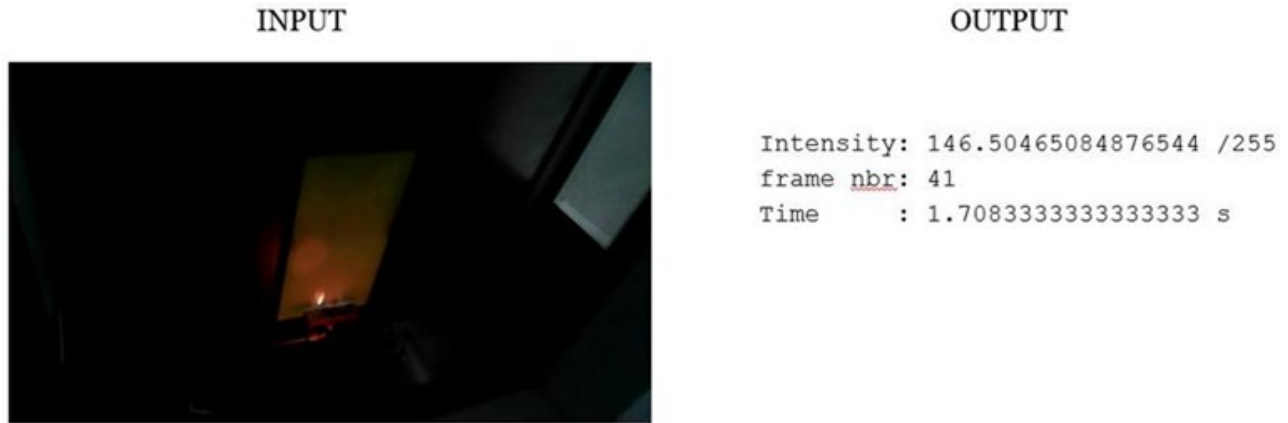
Figure 46: Light intensity extraction from flaming sample
