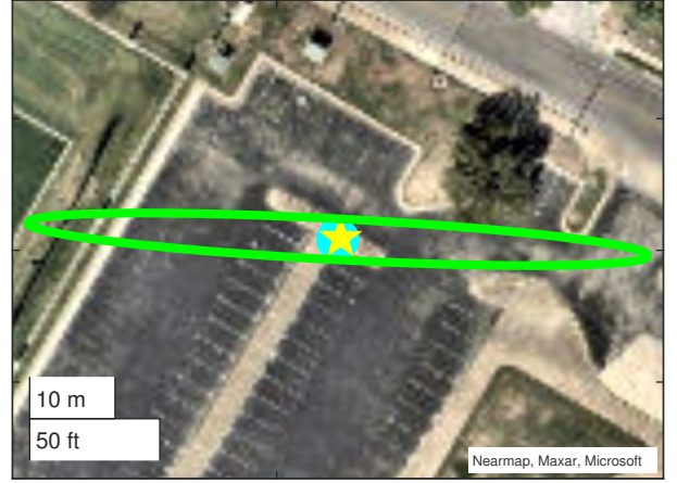
Fig. 9: Final UE position estimate, with the true position indicated with a star. The error of the final estimate is 0.35m, with the solution contained within a 95% error ellipse, which has a semi-major of 36.38m and a semi-minor of 2.40m.
