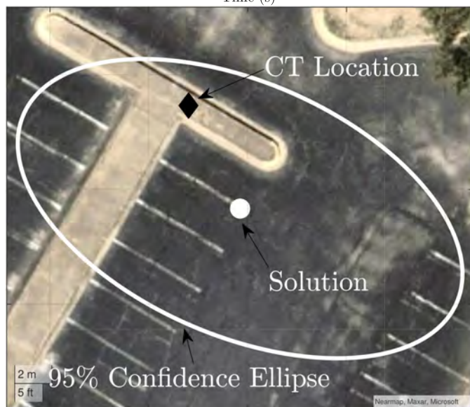
Fig. 7: The post-fit residuals from the NBLs estimator (top). The residuals are fairly zero-mean. Also plotted is the NBLs position solution, marked with a white circle, alongside the true location of the CT, marked with a black diamond. The solution has an absolute 3D error of 6.47 m, with a 95% confidence ellipse that has a semi-major axis of 11.96 m and a semi-minor axis of 6.31 m.
