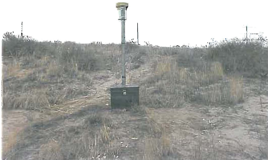
Figure 20. ATE 525WS rain gauge with 8-inch collector.
