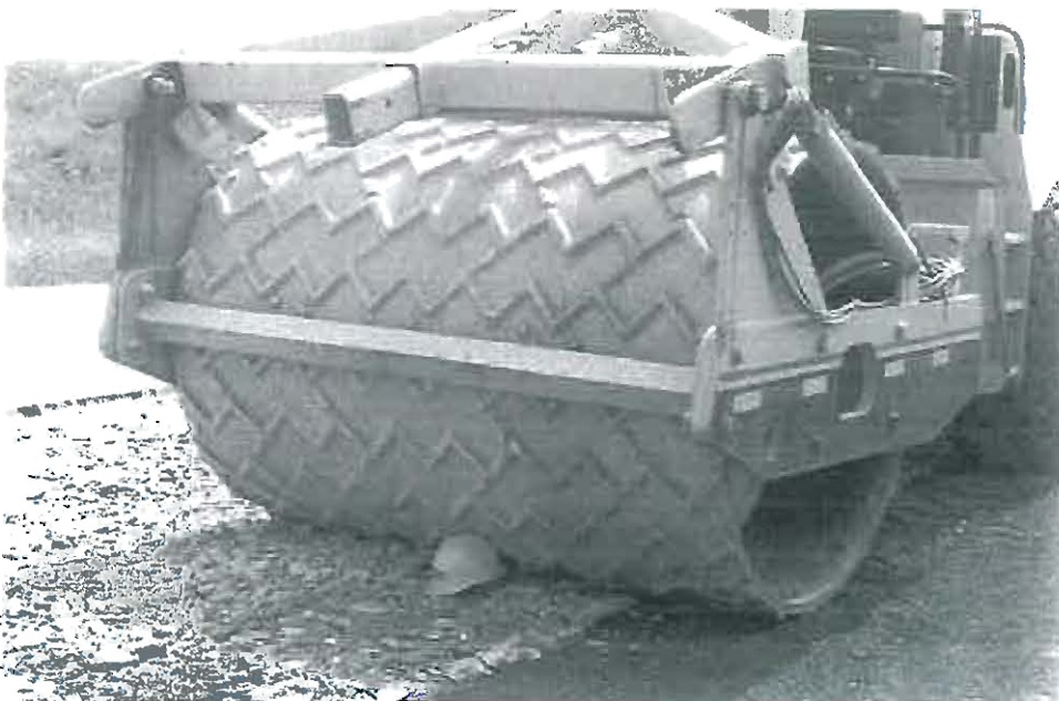
Figure 12. Steel vibratory roller with “Z” pattern grid on drum face was used to seat pavement.
