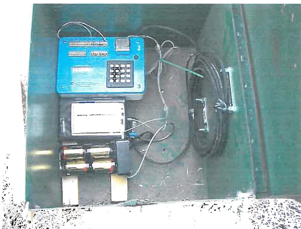
Figure 21. The Campbell Scientific CR21 datalogger is used to measure hourly rainfall.
