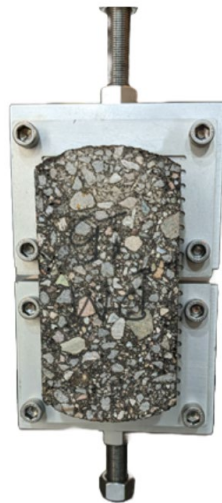
Figure A-18. Texas Overlay Tester Setup
