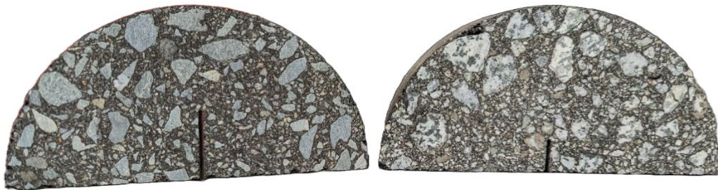
Figure A-16. LTRC-SCB Test Specimens
