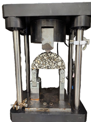
Figure A-15. Typical I-FIT Test Setup
