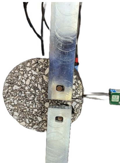
Figure A-12. Typical DCT Test Setup
