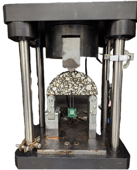
Figure A-13. Typical SCB Test Setup with CMOD Gauge
