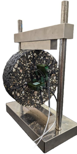
Figure A-14. Typical IDT Test Setup
