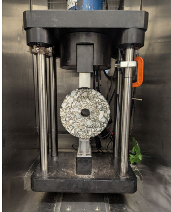
Figure 3: Loading Strips Embedded in an Axial Loading Device
