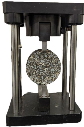
Figure A-21. Typical CT Index Test Setup
