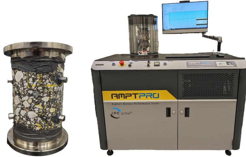
Figure A-17. AMPT Cyclic Fatigue Test Specimen and Setup
