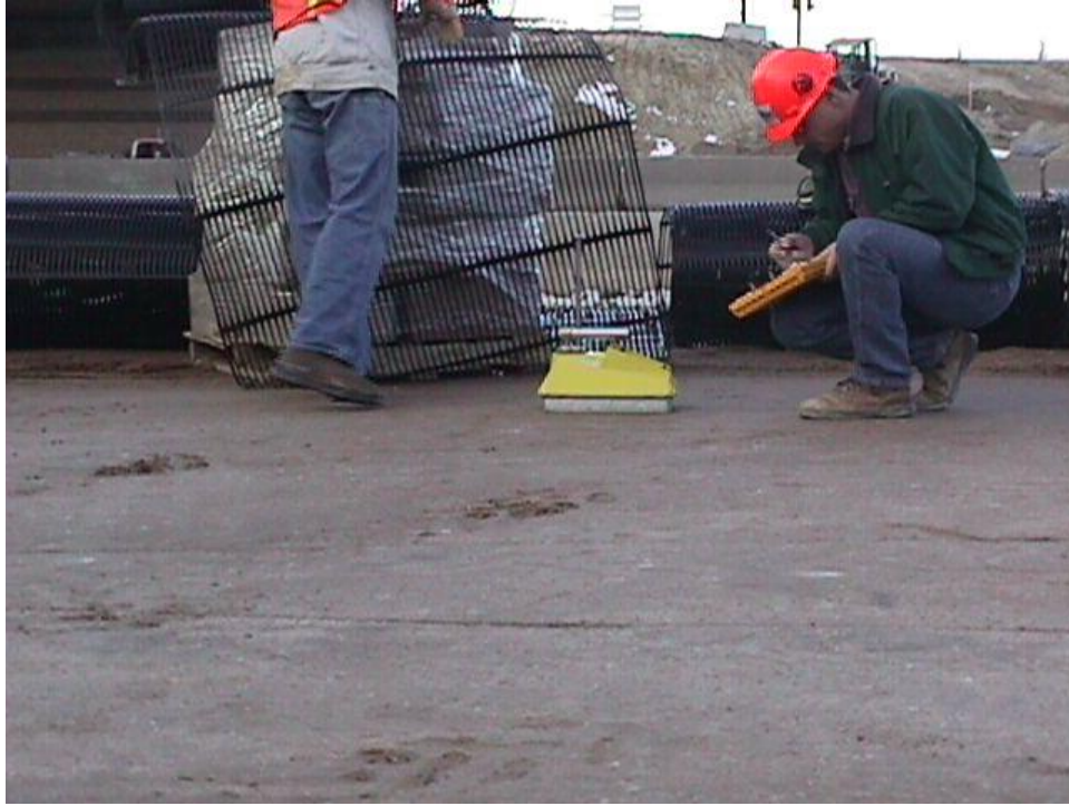
Figure B-15. Backfill levels of compaction were checked with a nuclear gage.
