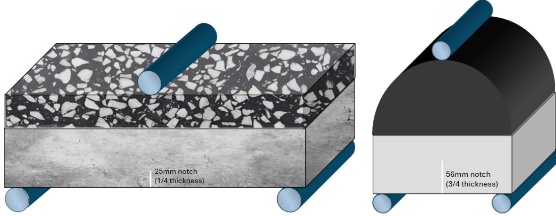
Figure 8. Three-dimensional finite element models and loading configurations used for the numerical simulation of the (a) rectangular and (b) semi-cylindrical pavement specimens.
