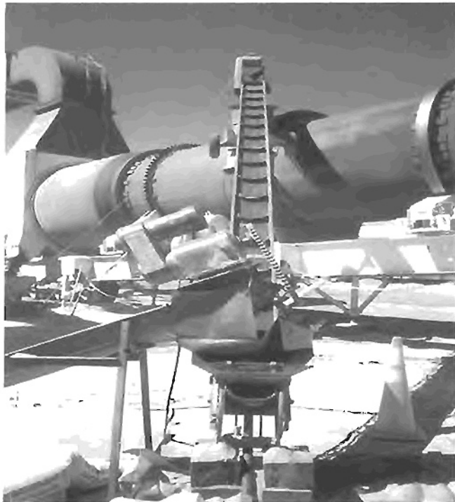
Figure 6. Conveyor system used to add Vestoplast S and fiber pellets at the RAP collar.
