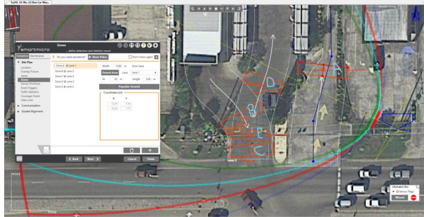
Figure 55. Counting locations for the oblique positioning of the radar device at the car wash site, July 11-14, 2024
