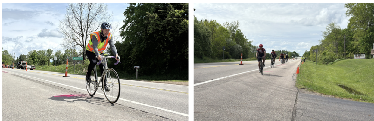
Figure 21. Bicyclists Contacting Rumble Strips during Test Rides
