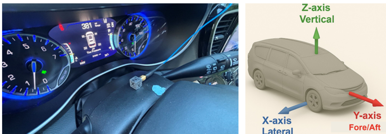
Figure 11. Triaxial Accelerometer Position on Steering Column (left) and Orientation (right)
