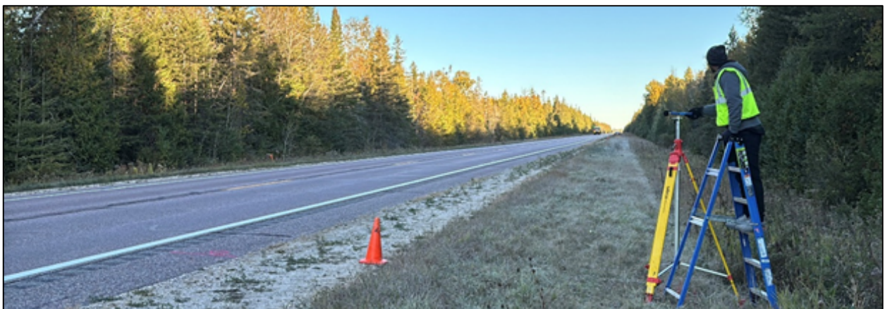
Figure 9. Roadside Noise Measurement Setup
