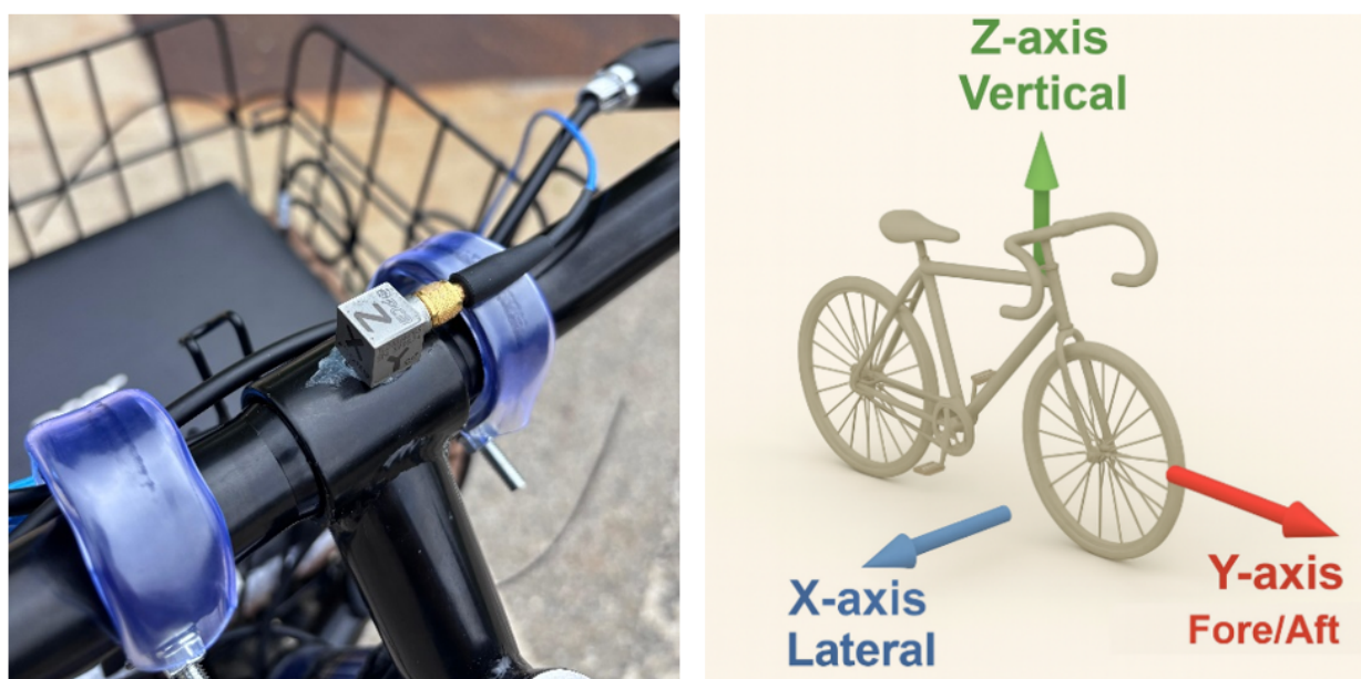
Figure 22. Triaxial Accelerometer Position on Handlebar (left) and Orientation (right)
