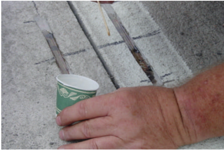
Figure 23. Attaching Strain Gages using Fast-Setting Epoxy
