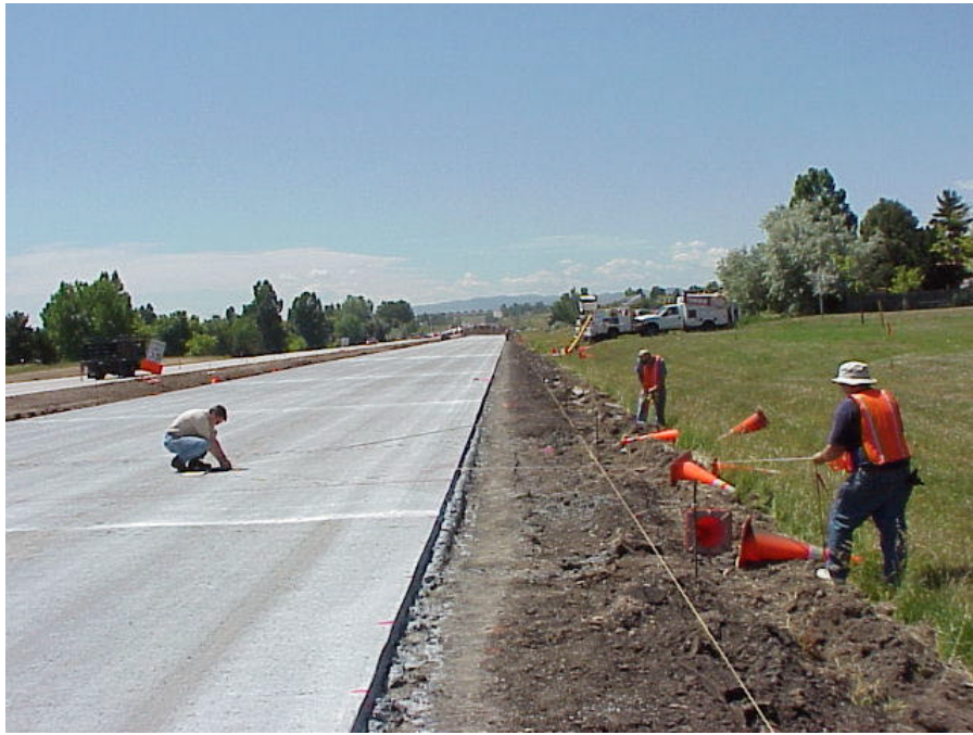
Figure 21. Determination of Surface Gage Locations from the Reference Points
