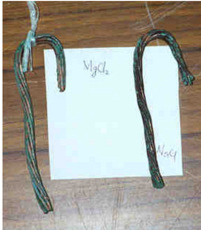
Figure 14: Corroded copper wires after SAE J2334 testing
