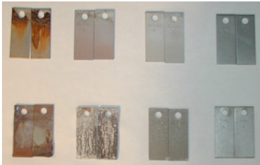
Fig. 2-16 Coupons after the NACE test
