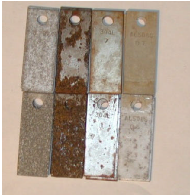
Fig.2-17 Coupons after the SAE test (Upper: exposed to the NaCl solution, lower: exposed to the \text{MgCl}_2 solution)
