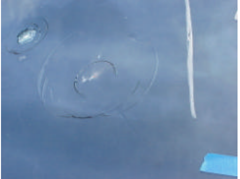
Figure 13 Bulls-eye pattern damage
