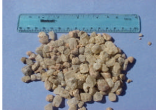
d) Quartz sample used in Test A
