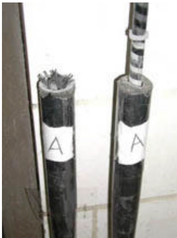
Figure 21: Uncond. CFRP Failure
