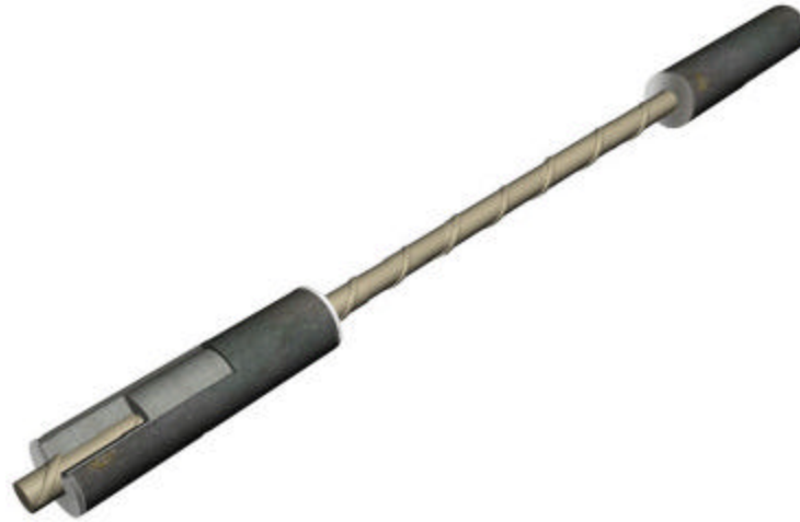
Figure 9: 3-D View of Bar and Anchor Layout
