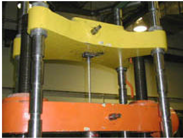
Figure 17: 24-Inch FRP Bar in Tensile Testing Apparatus
