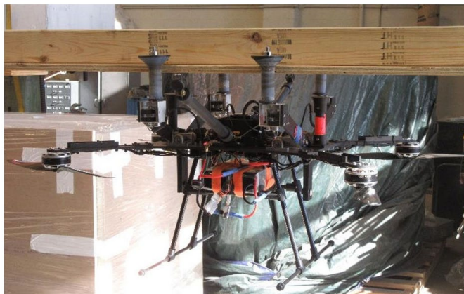
Figure 6. Photo. Demonstration of a UAS designed for close-up inspection.
