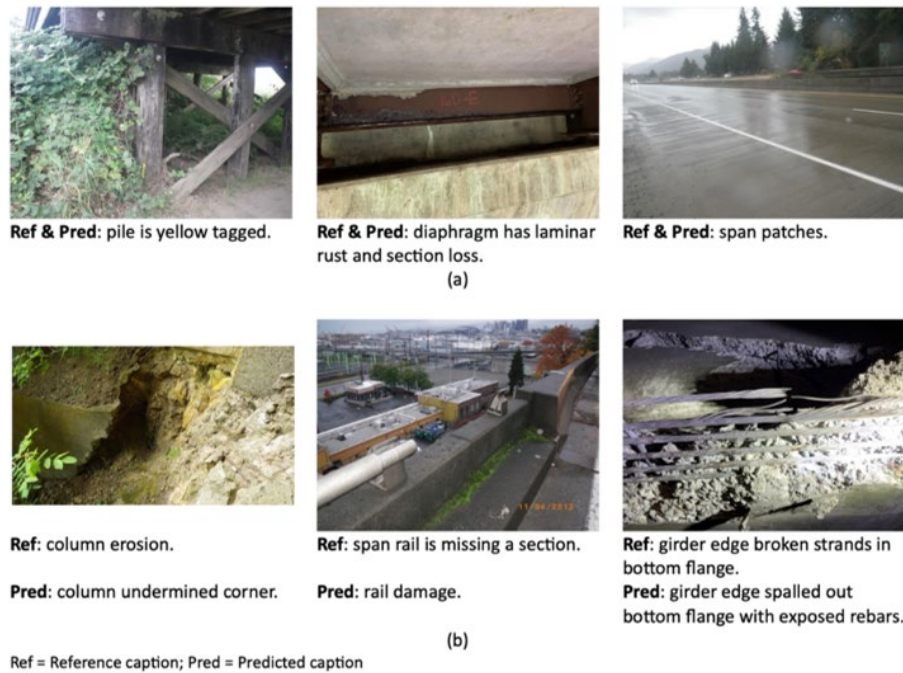
Figure 25. Illustration. Examples of inspection image captioning using vision-language models.
