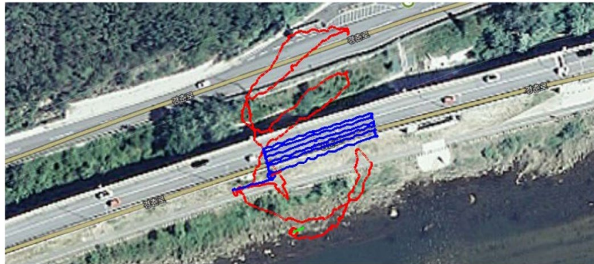
Figure 19. Graph. Comparison of trajectories estimated using GNSS (red) and LiDAR-based SLAM (blue).
