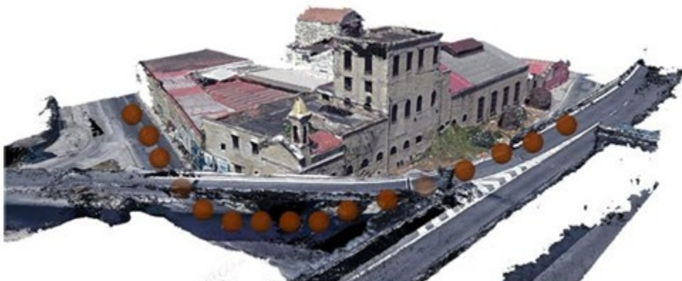
Figure 27. Point cloud visualization. Demonstration of urban scene reconstruction using 360-degree images.
