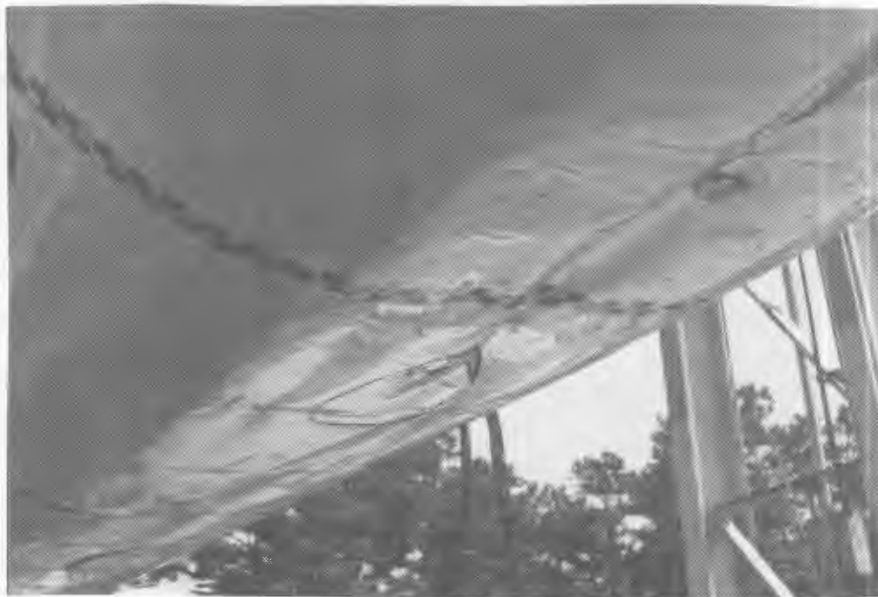
FIGURE 57. POST TEST UNDERSIDE FUSELAGE DAMAGE - 2
