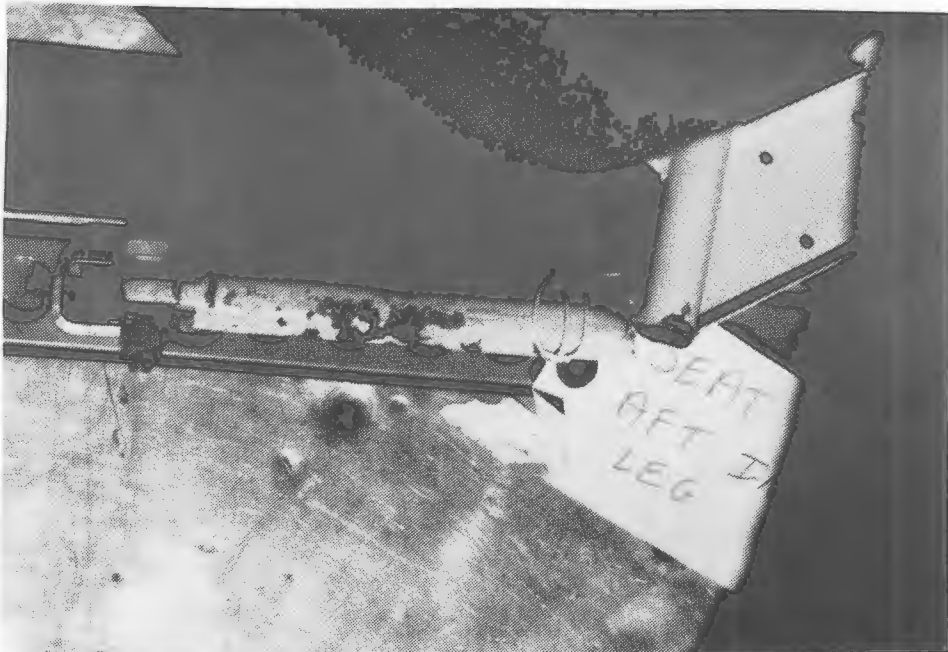
FIGURE 21. POST TEST SEAT 3, INBOARD AFT LEG
