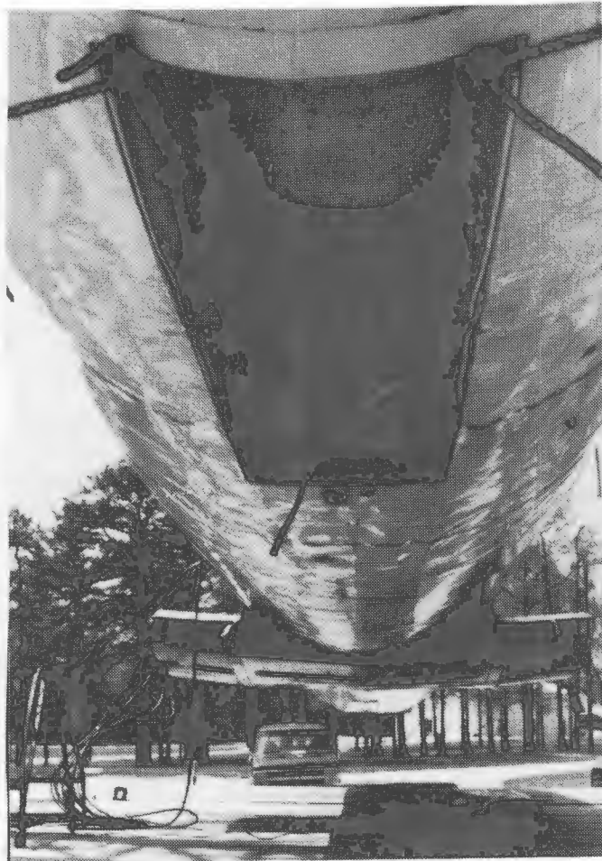
FIGURE 56. POST TEST UNDERSIDE FUSELAGE DAMAGE - 1
