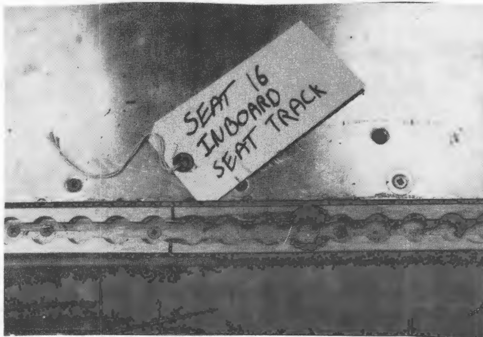
FIGURE 55. POST TEST SEAT TRACK, SEAT TRACK
