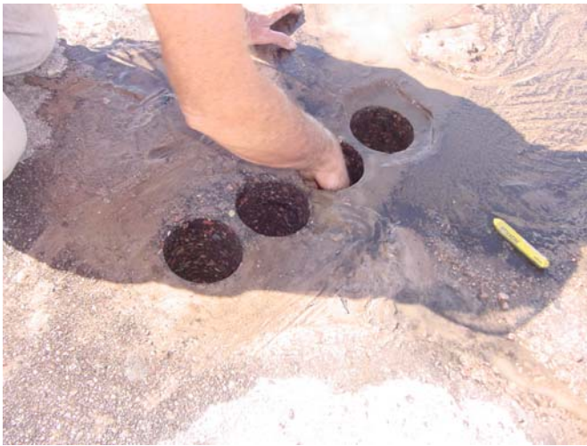
Figure 20 - In order to determine the lateral extent of stripping, additional cores were obtained at six-inch intervals transversely to the construction joint.
