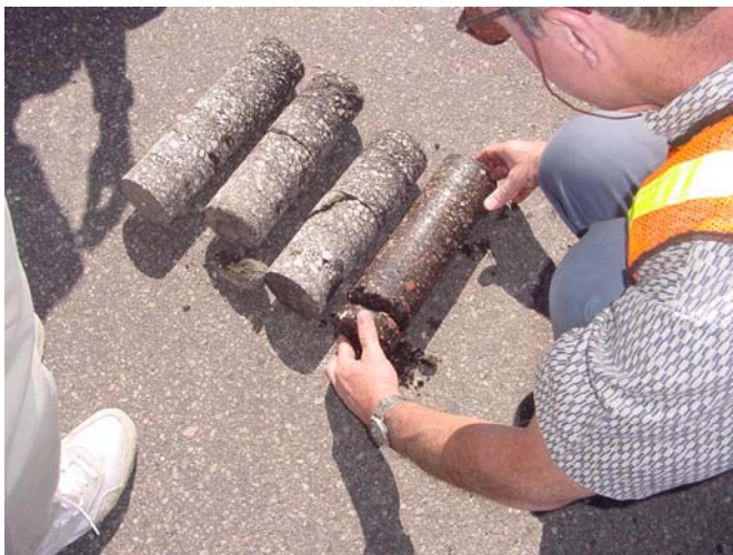
Figure 21 - It is apparent from this picture that the stripping occurs only immediately at the joint. Only the core sample right over the construction joint (right core) has evidence of stripping.
