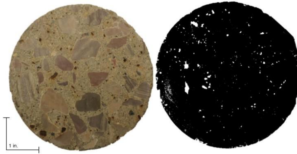
Figure 30: SDSMT Sample: 8% Air Content*
