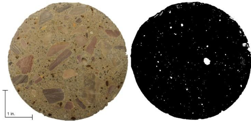
Figure 29: SDSMT Sample: 5% Air Content
