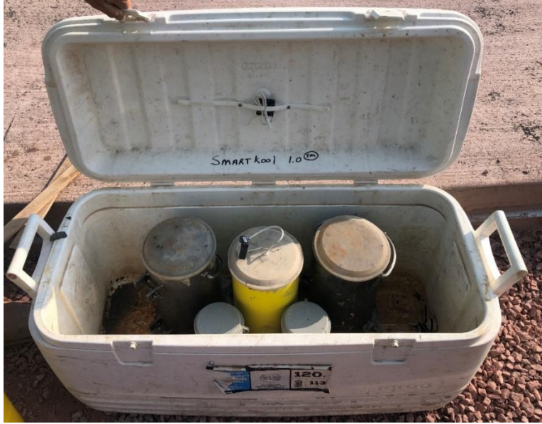
Figure 4: Cooler with concrete cylinder samples and sensors
