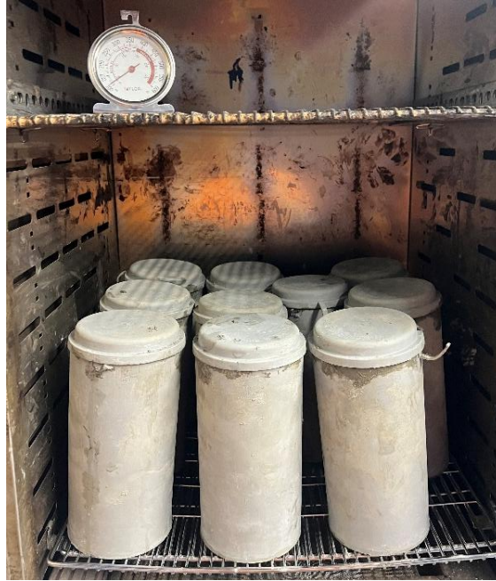
Figure 7: Cylinder configuration in oven
