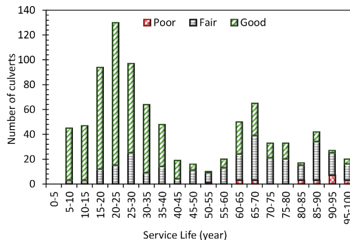
Figure 5.31: CIP RCBCs Condition Ratings vs. Service Life.
