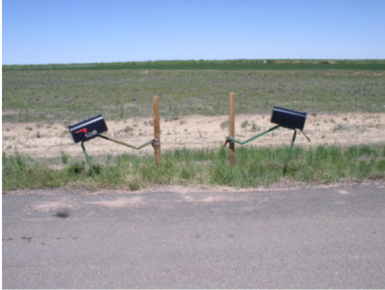
Figure 3. The Roadside Safety Devices mounting system does not reliably return to the centered position.
