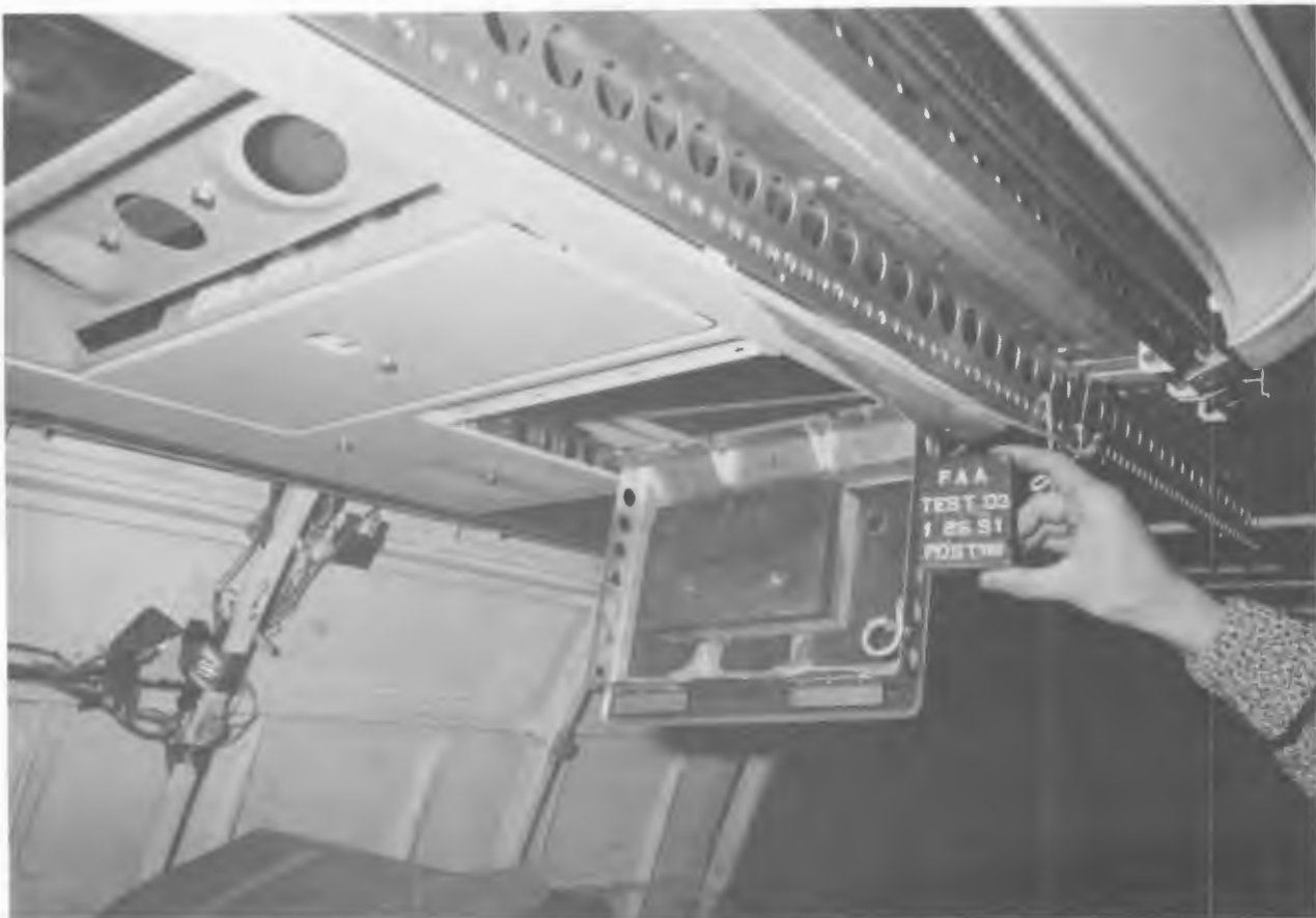
Figure 132. POST-TEST BIN 'B' FORWARD UNDERSIDE PANEL ACCESS DOOR
