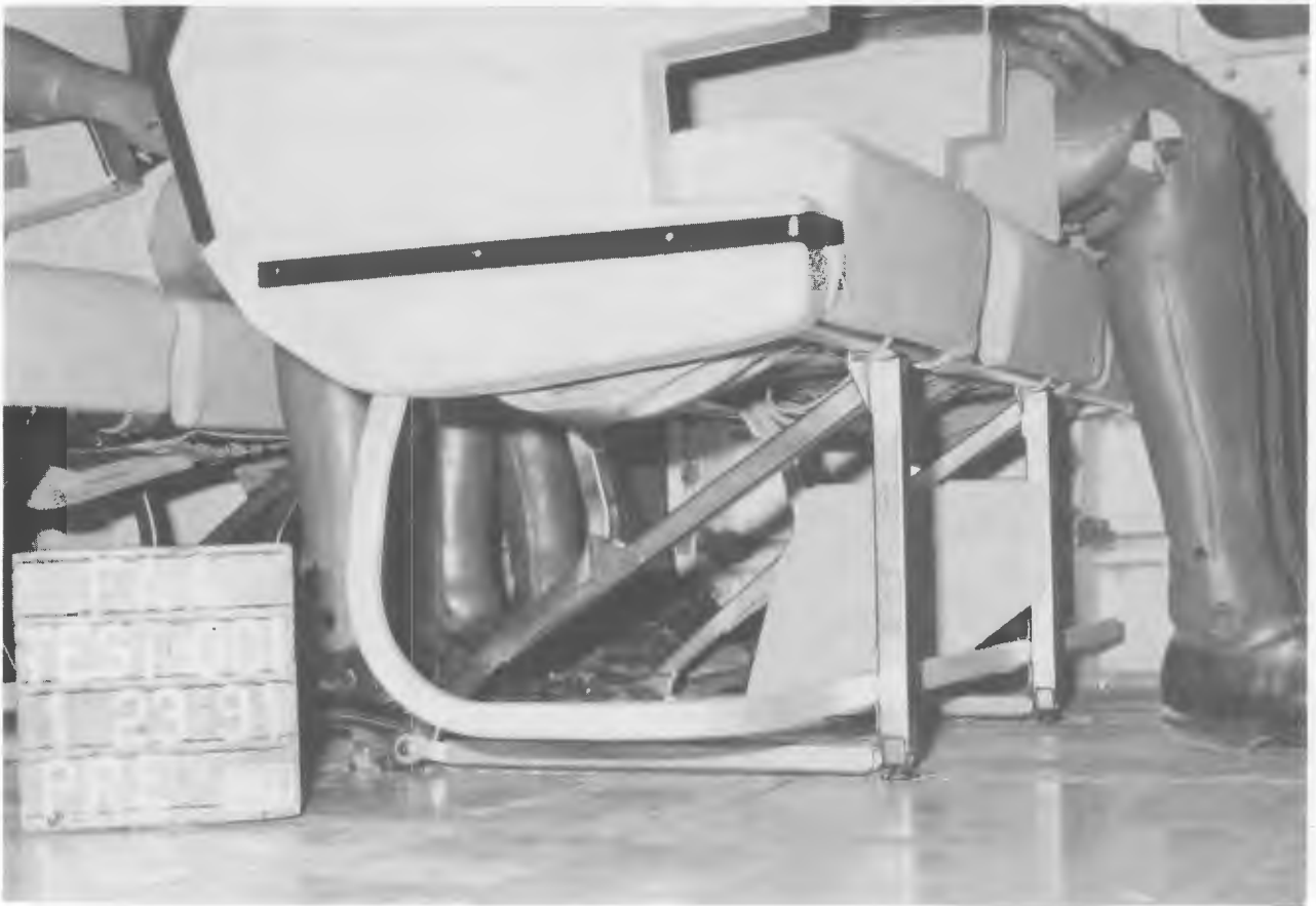
Figure 36. PRE-TEST FRONT SEAT/FLOOR ATTACHMENT
