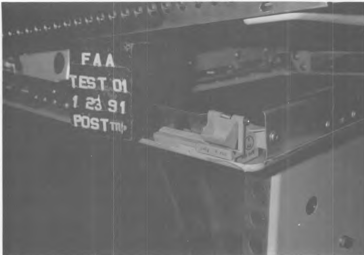
Figure 44. POST-TEST BIN 'B' FORWARD UNDERSIDE PANEL-FWD. LATCH CLOSE-UP
