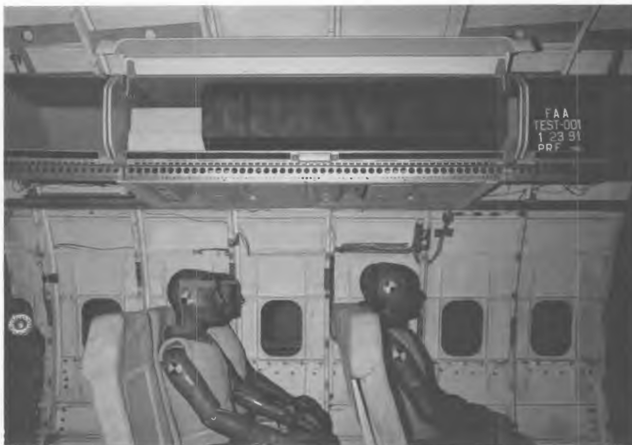
Figure 13. PRE-TEST BIN 'B' BALLAST POSITION
