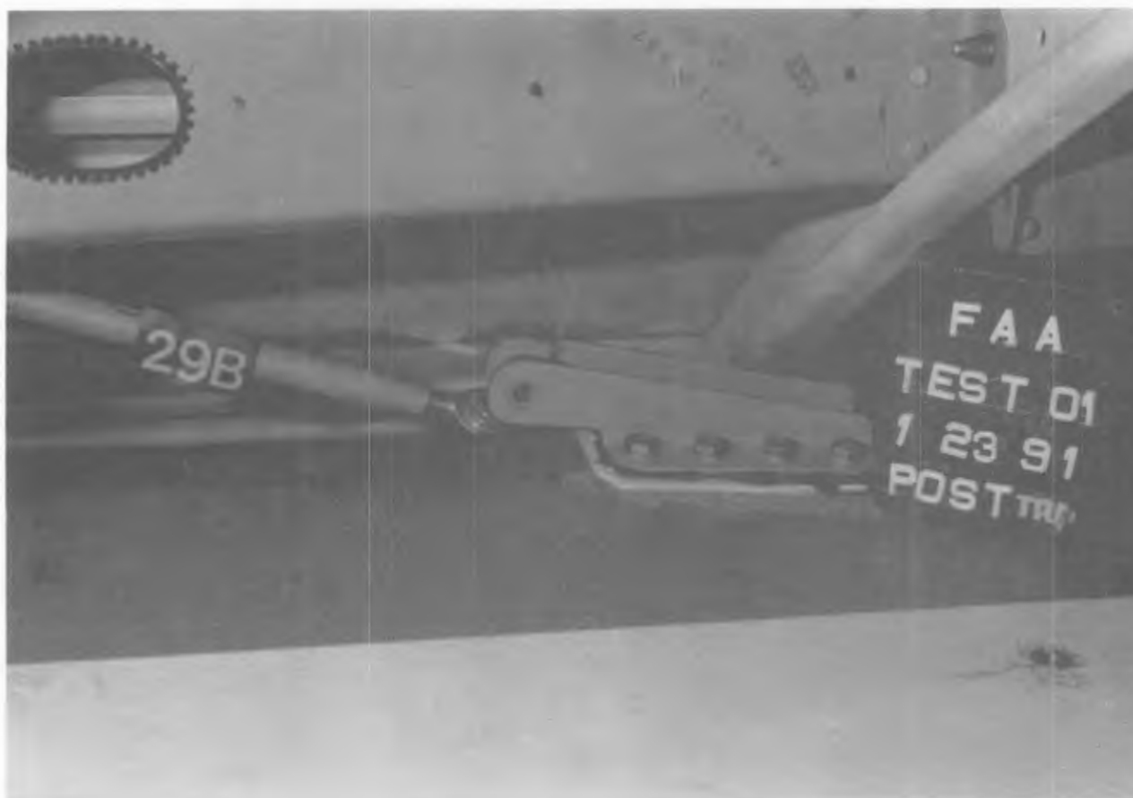
Figure 57. POST-TEST BIN 'B' REAR 20" BIN DRAG LINK FITTING/FUSELAGE CONTACT
