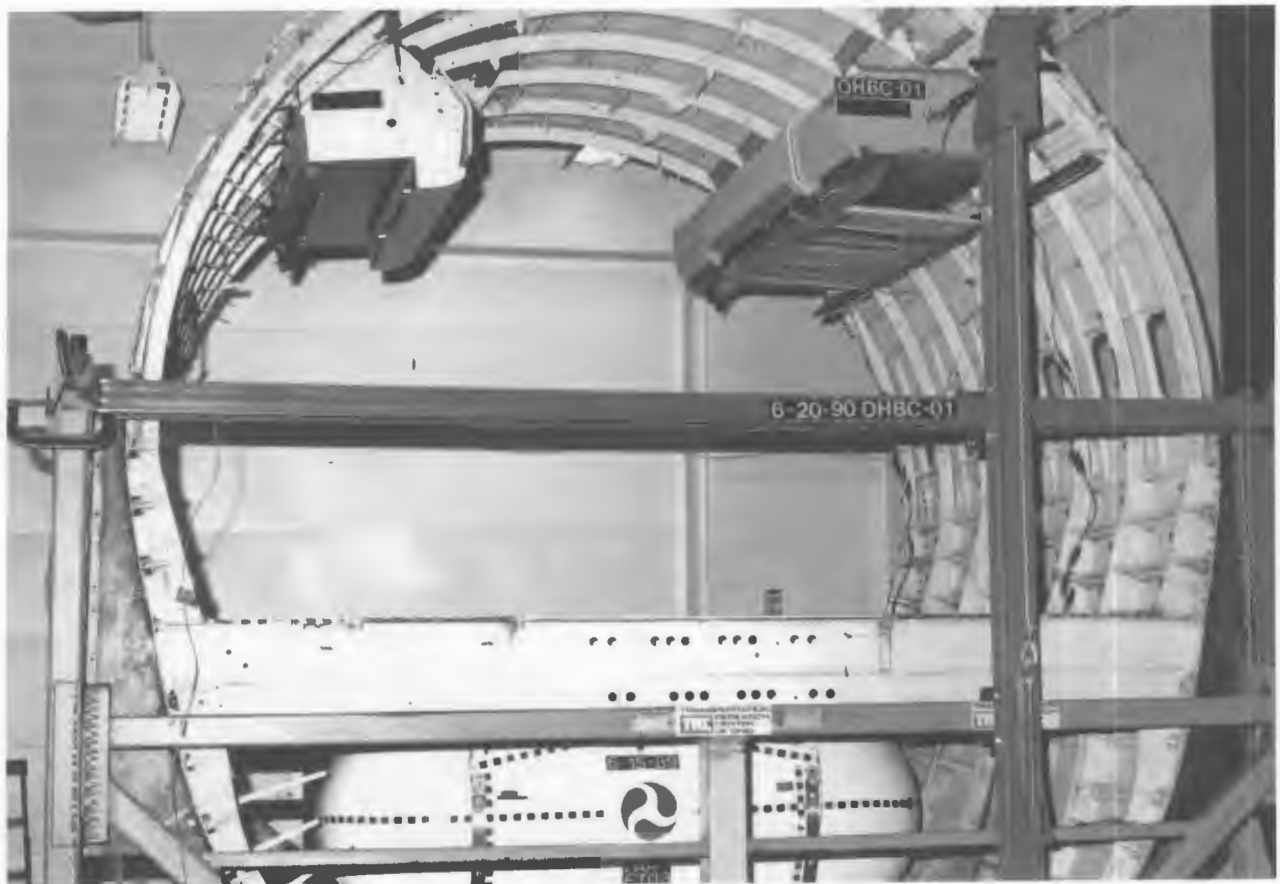
Figure C-4. FRONT VIEW OF FUSELAGE AND STATIC TEST FIXTURE, TEST OHBC-01
