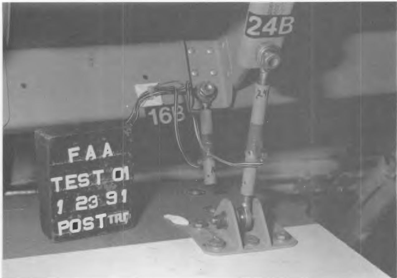
Figure 48. POST-TEST BIN 'B' LINKS 16 AND 24
