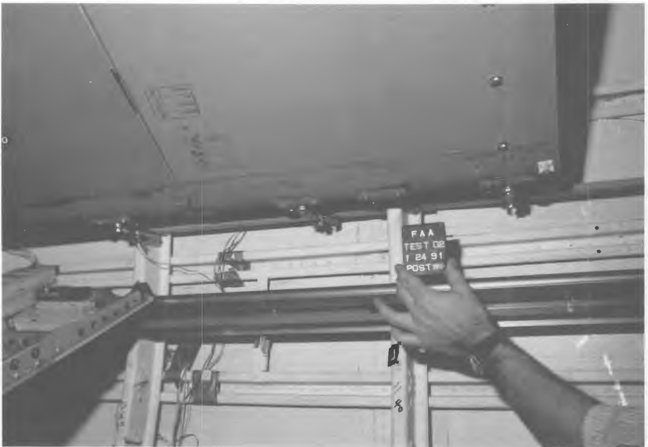
Figure 97. POST-TEST BIN 'B' FORWARD LOWER LATERAL LINKS
