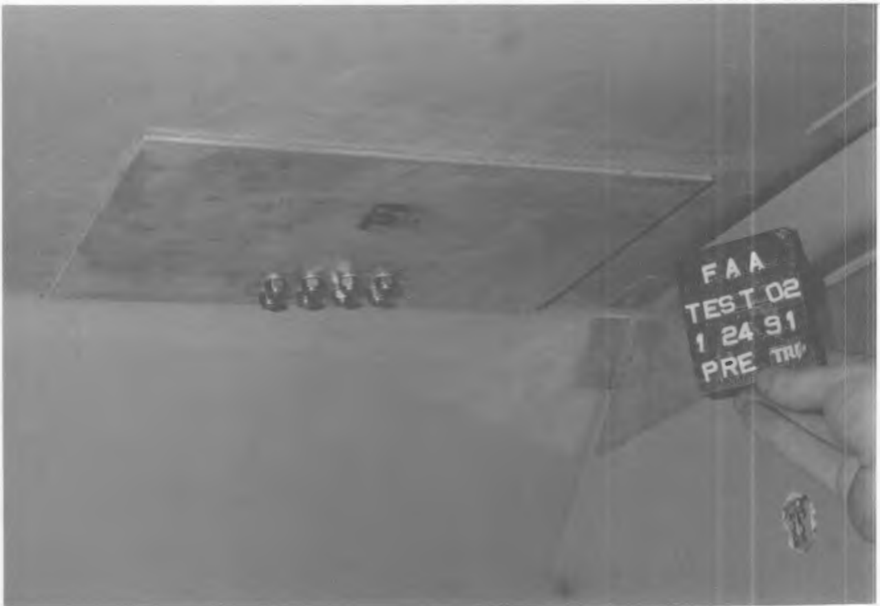
Figure 87. PRE-TEST BIN 'B' 60" BIN DRAG LINK MOUNT INTERIOR REINFORCEMENT PLATE
