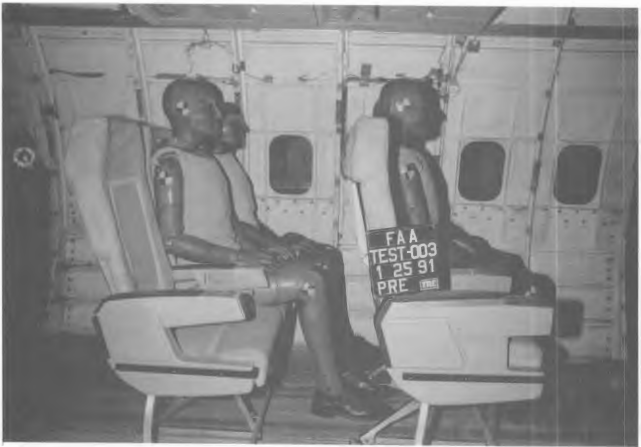
Figure 125. PRE-TEST SEATS AND DUMMIES SIDE VIEW
