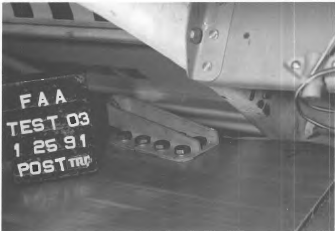
Figure 146. POST-TEST BIN 'B' 60" BIN DRAG LINK FITTING/FUSELAGE CONTACT FRONT ANGLE VIEW
