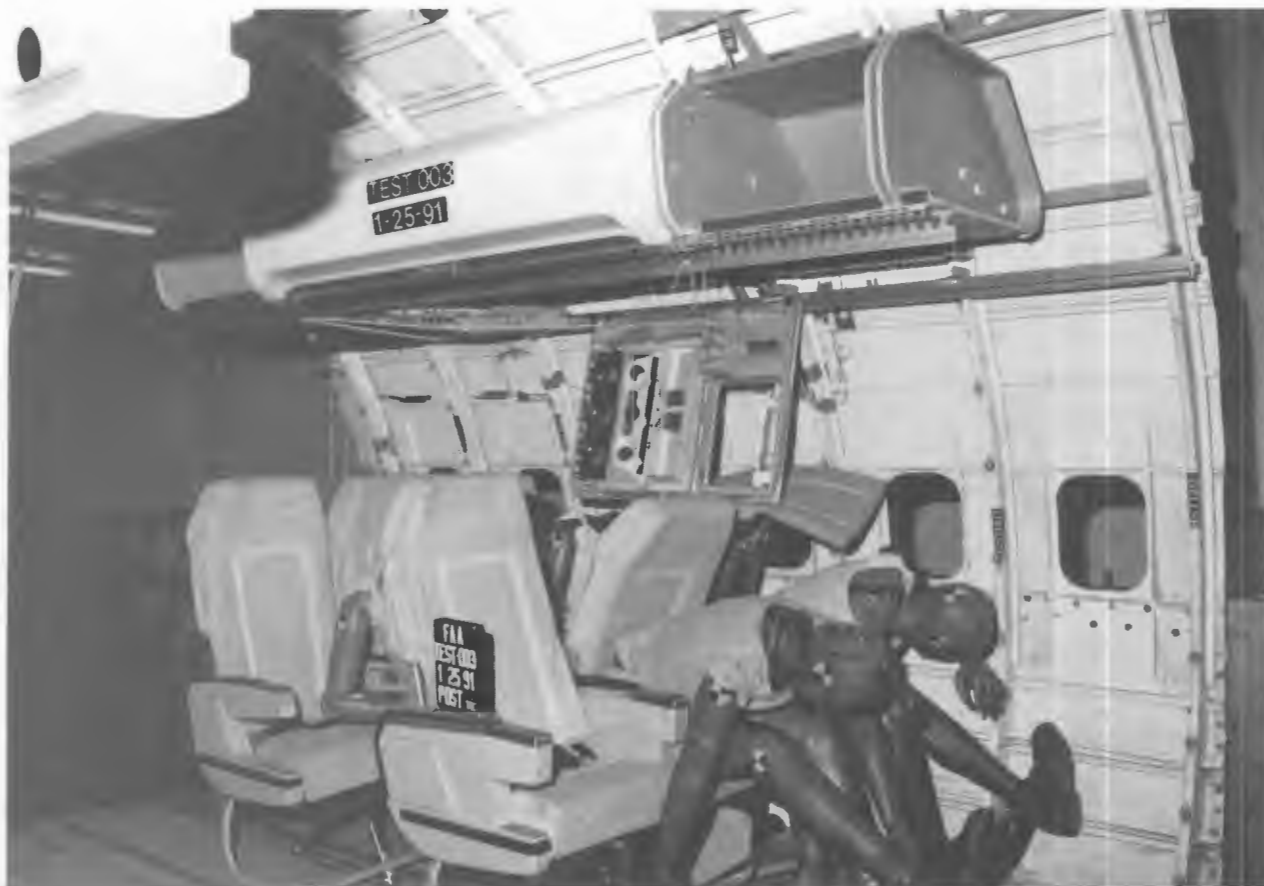
Figure 161. POST-TEST SEATS, DUMMIES, AND BIN 'B' FRONT ANGLE VIEW
