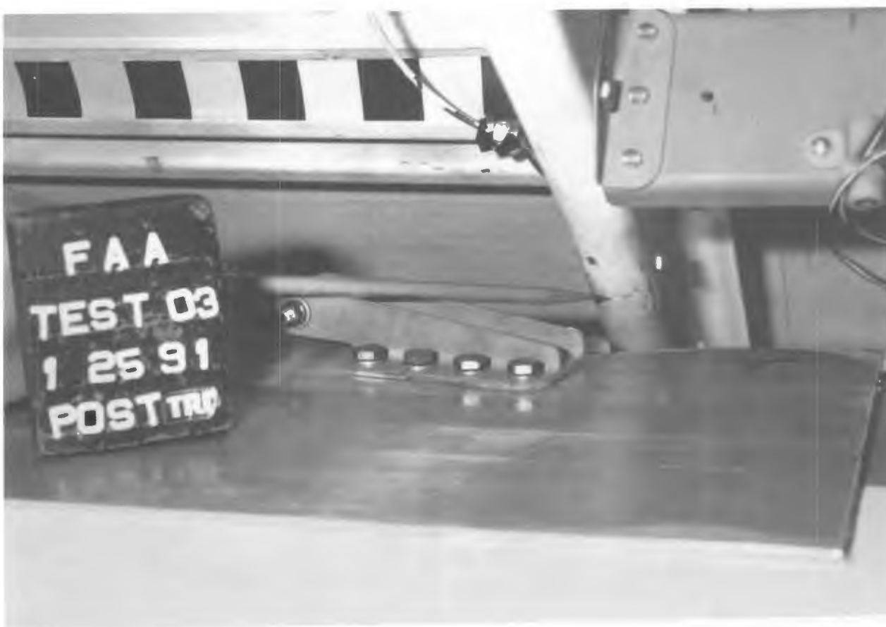
Figure 148. POST-TEST BIN 'B' 60" BIN DRAG LINK FITTING/FUSELAGE CONTACT, LOWER MARKS ON FUSELAGE
