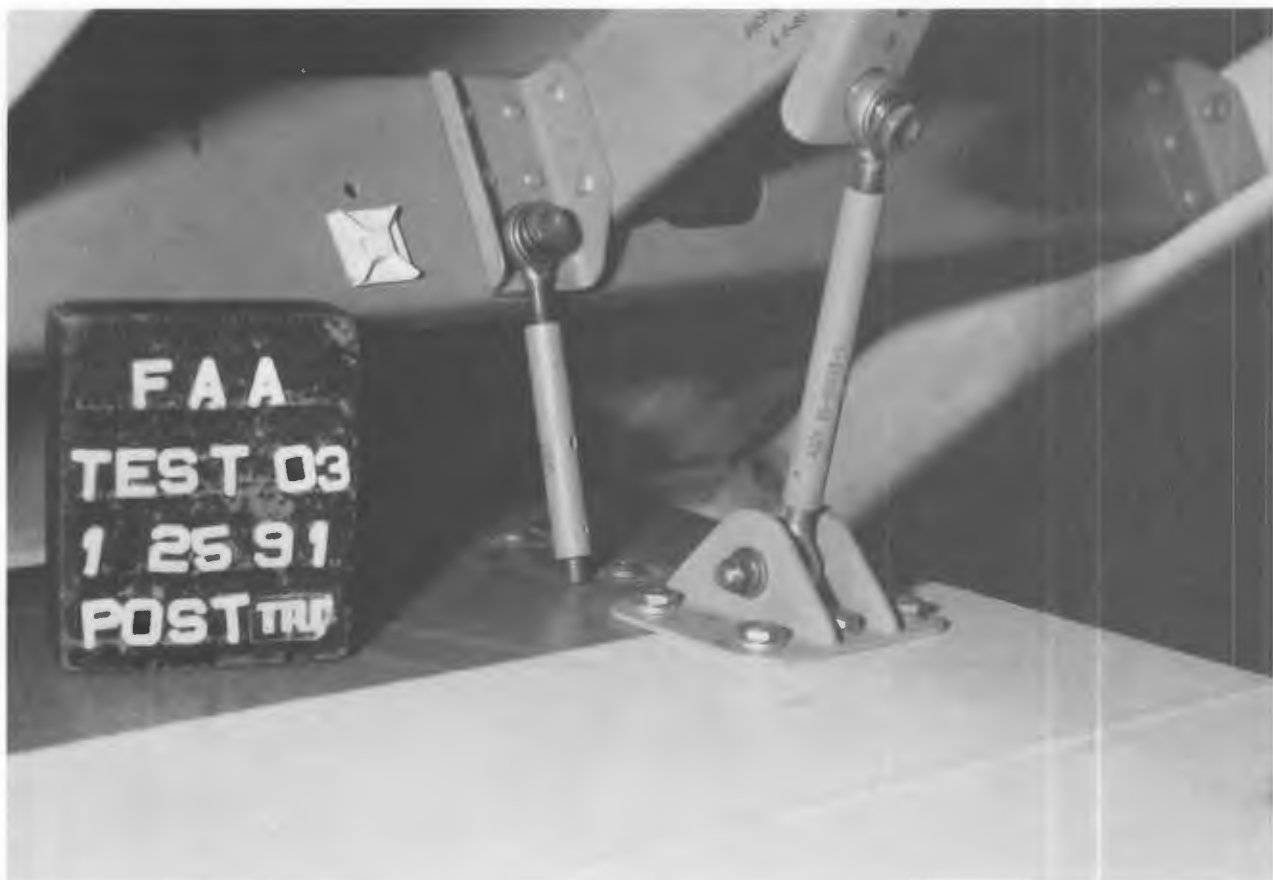
Figure 138. POST-TEST BIN 'B' FORWARD UPPER LINKS
