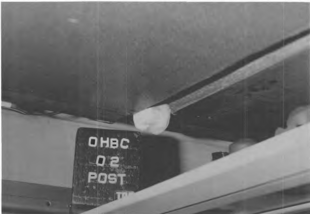
Figure C-23. POST-TEST OHBC-02, BIN 'B' OUTBOARD DEFLECTION INDICATOR BETWEEN THE 60" BIN AND REAR 20" BIN
