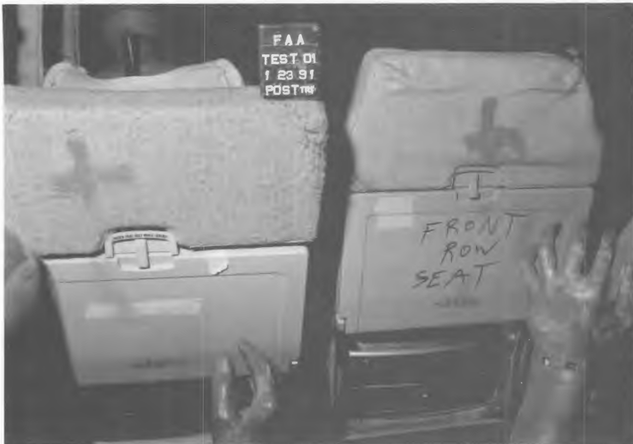
Figure 68. POST-TEST REAR DUMMY CONTACT WITH FRONT SEAT
