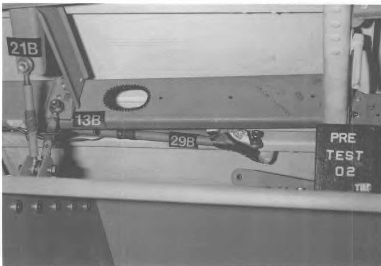
Figure C-19. PRE-TEST OHBC-02, BIN 'B' LINK 29 DETACHED C-20
