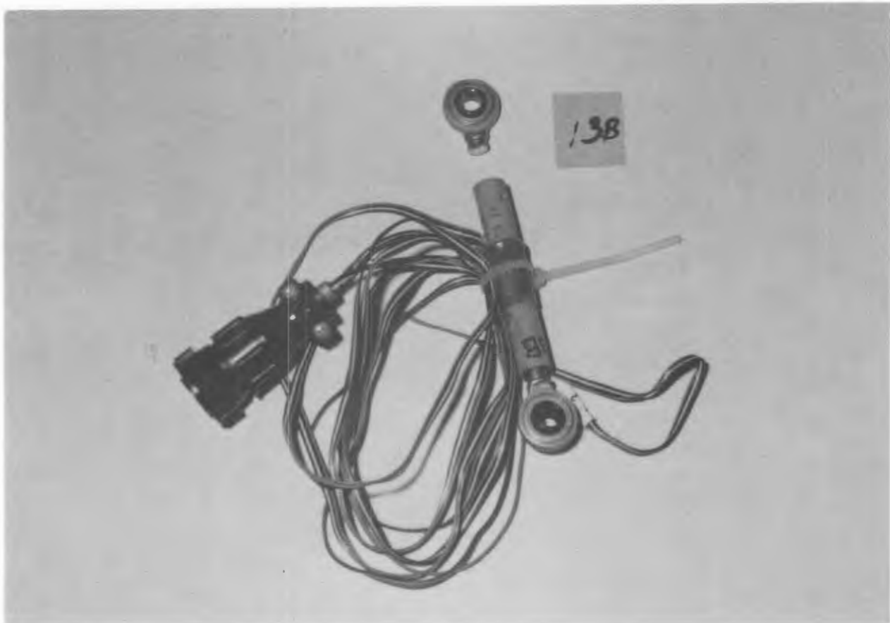
Figure 73. POST-TEST BIN 'B' LINK 13 CLOSE-UP REMOVED FROM TEST FIXTURE
