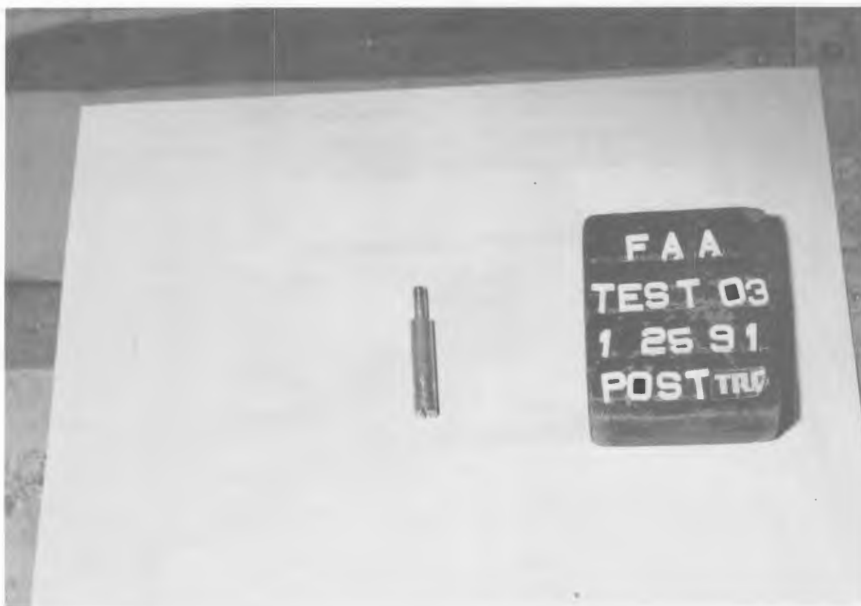
Figure 160. POST-TEST BIN 'A' REAR SUPPORT BAR SHEAR PIN, REMOVED
