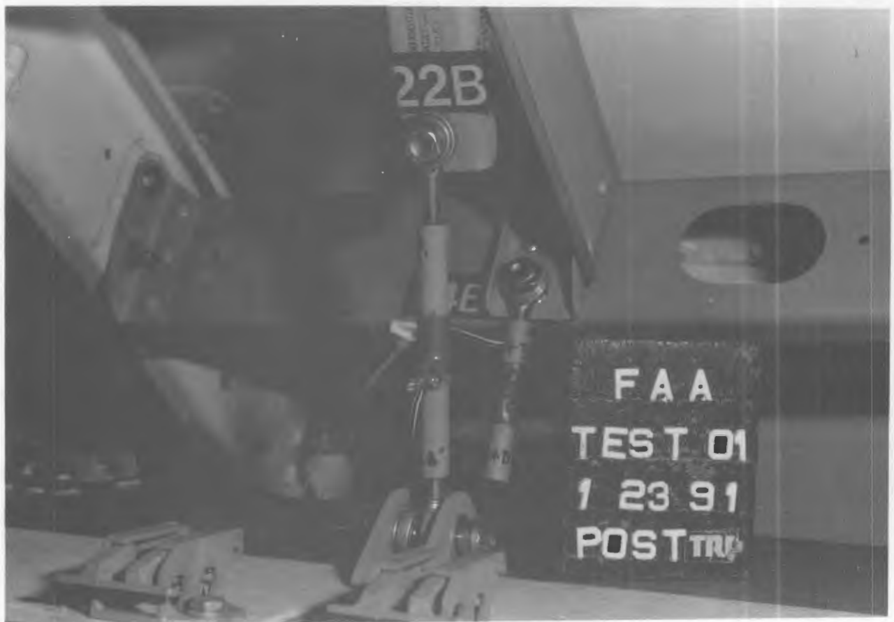
Figure 55. POST-TEST BIN 'B' LINKS 14 AND 22
