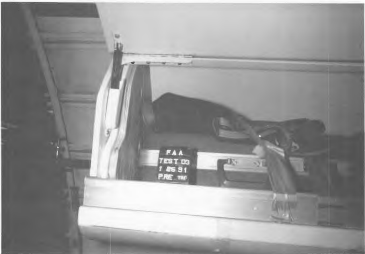
Figure 123. PRE-TEST BIN 'A' FOAM/WOOD LOAD DISTRIBUTORS
