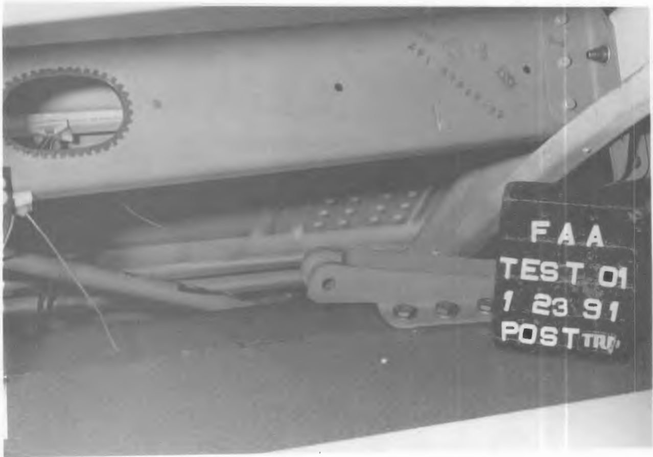
Figure 50. POST-TEST BIN 'B' FORWARD 20" BIN DRAG LINK FITTING/FUSELAGE CONTACT
