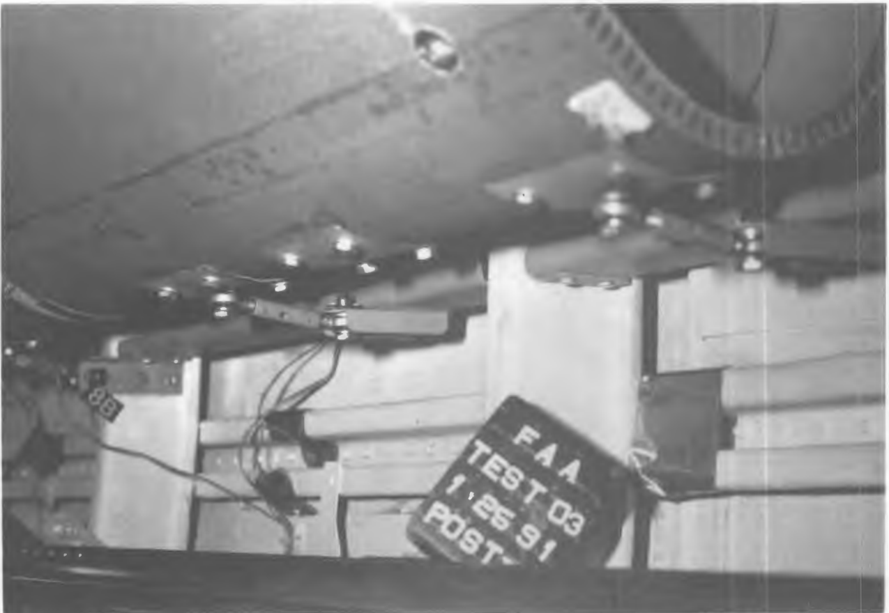
Figure 134. POST-TEST BIN 'B' FORWARD LOWER LATERAL LINKS
