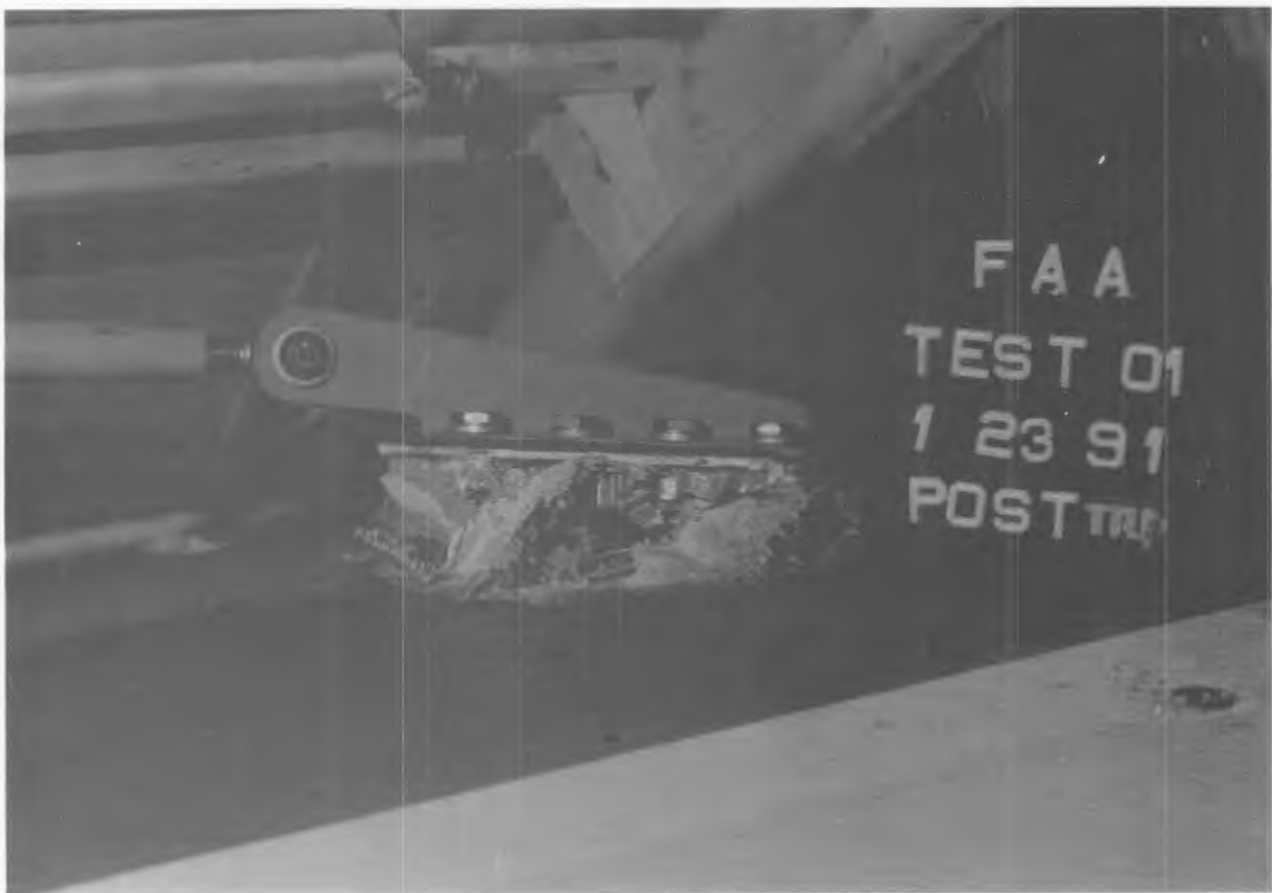
Figure 53. POST-TEST BIN 'B' LINK 32 BIN ATTACHMENT
