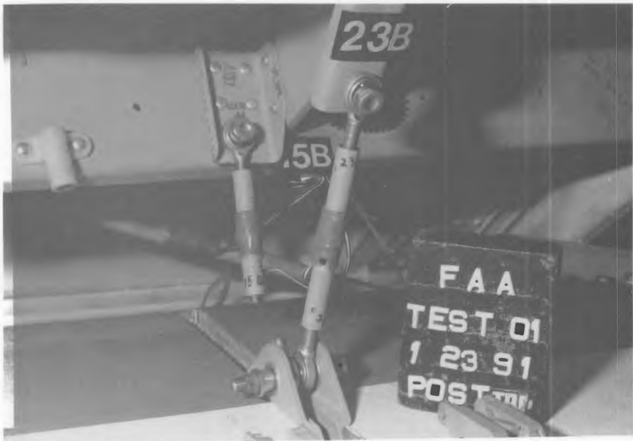
Figure 51. POST-TEST BIN 'B' LINKS 15 AND 23
