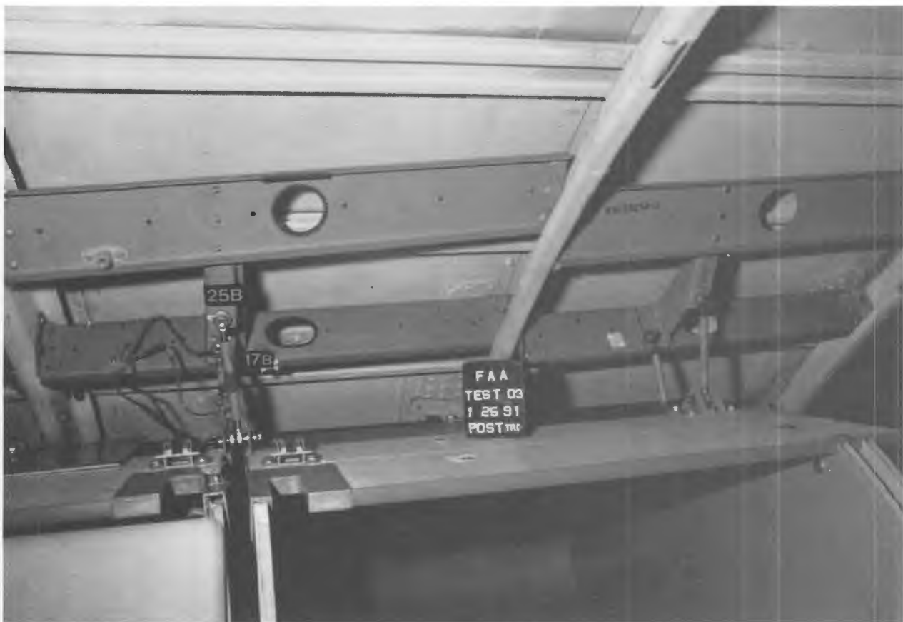
Figure 137. POST-TEST BIN 'B' LINKS 17, 25, AND FORWARD UPPER LINKS
