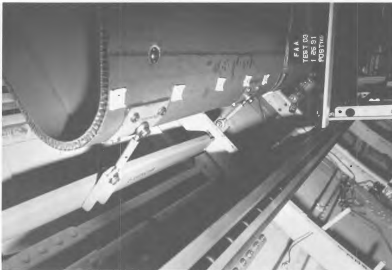
Figure 136. POST-TEST BIN 'B' REAR LOWER LATERAL LINKS
