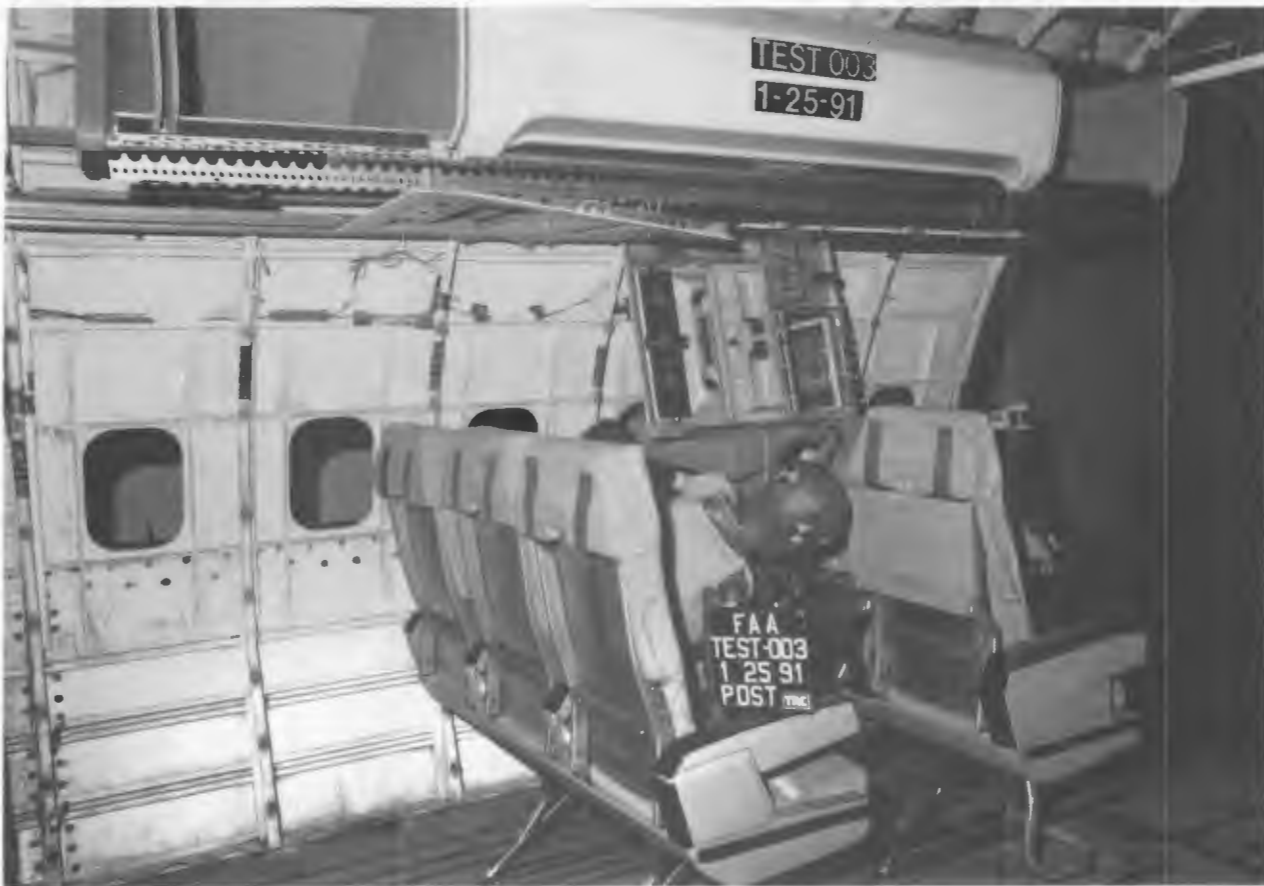
Figure 163. POST-TEST SEATS AND DUMMIES REAR ANGLE VIEW
