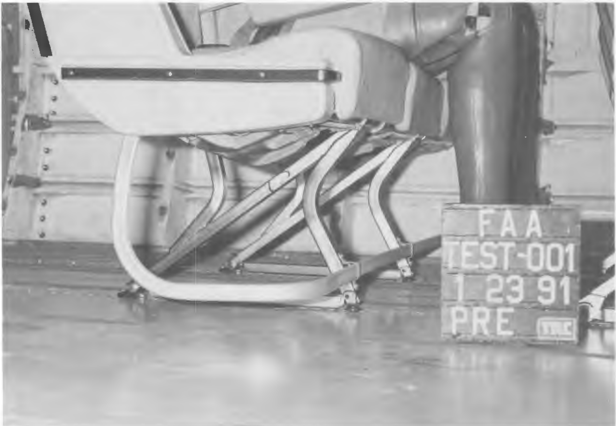
Figure 37. PRE TEST REAR SEAT/FLOOR ATTACHMENT
