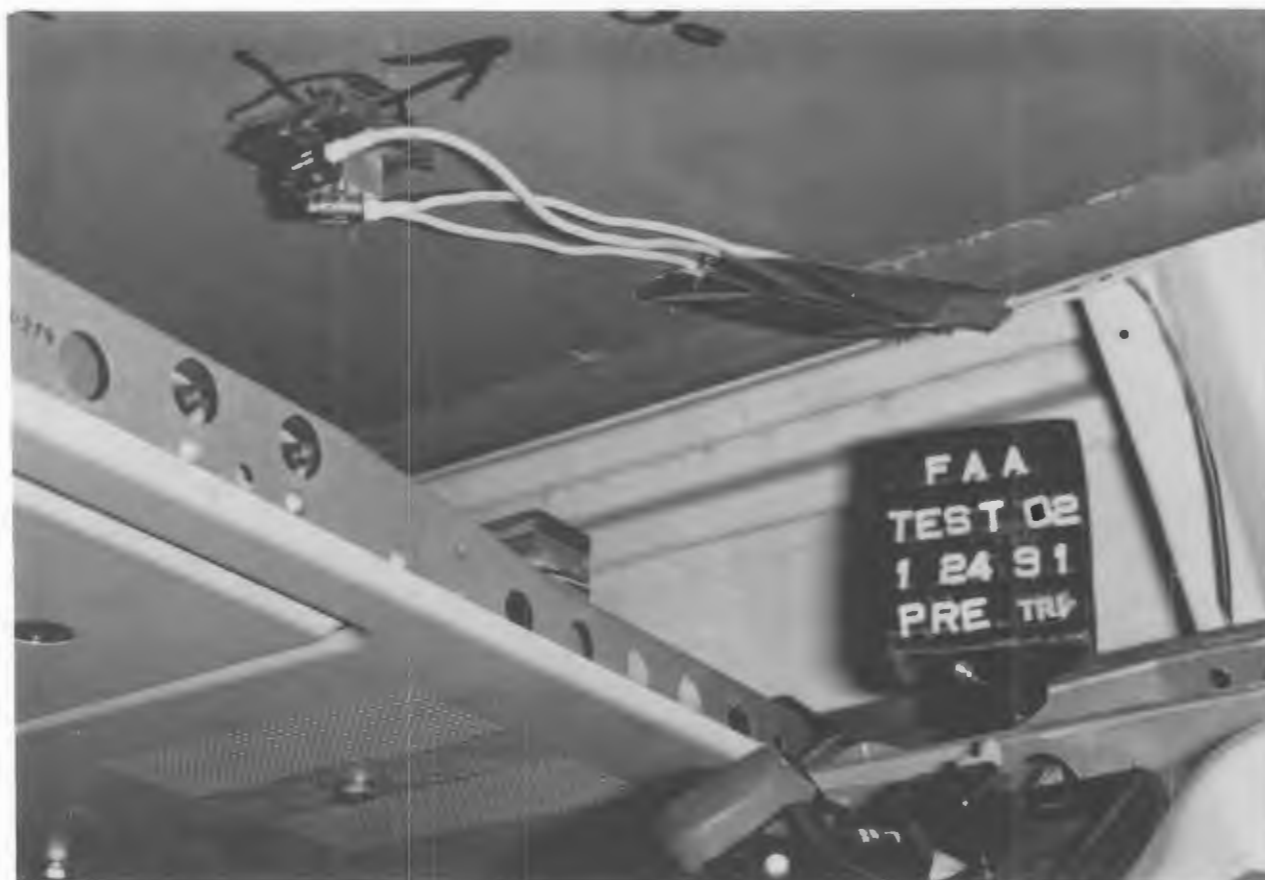
Figure 82. PRE-TEST BIN 'B' ACCELEROMETER POSITION
