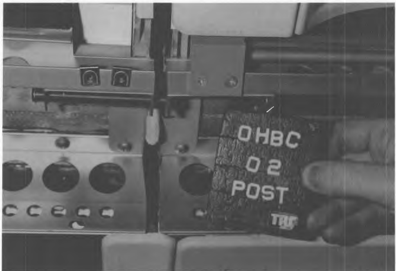
Figure C-21. POST-TEST OHBC-02, BIN 'B' INBOARD DEFLECTION INDICATOR BETWEEN THE 60" BIN AND REAR 20" BIN
