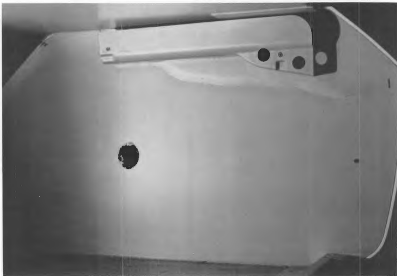
Figure C-15. POST-TEST OHBC-01 DAMAGE, 60" BIN FORWARD PANEL C-18
