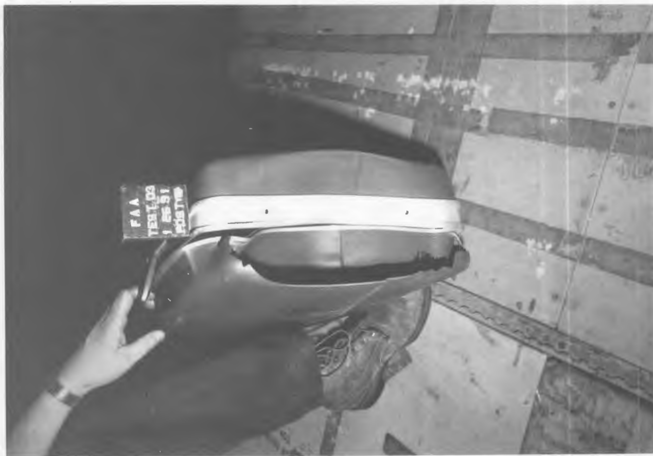
Figure 154. POST-TEST BIN 'A' BALLAST DAMAGE
