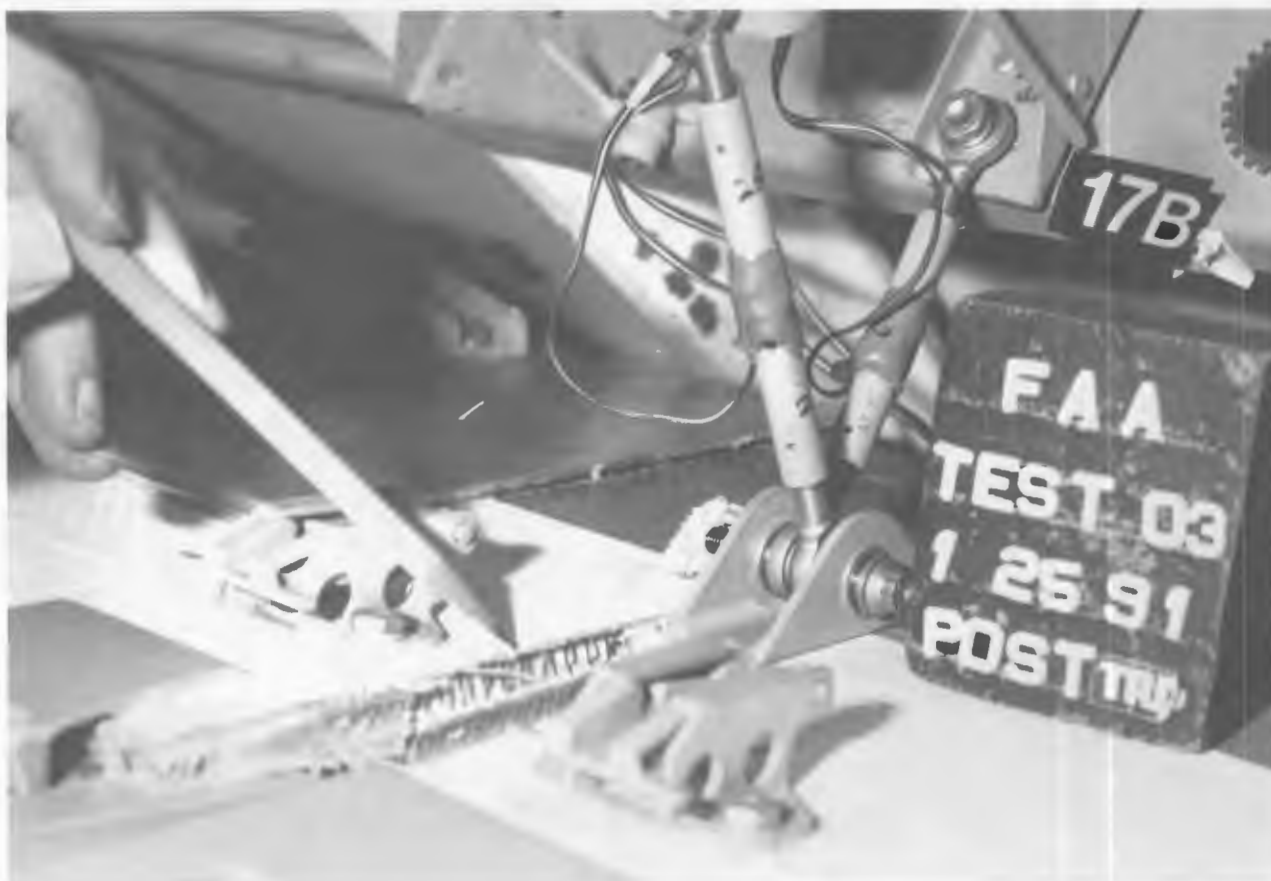
Figure 142. POST-TEST BIN 'B' 60" BIN FORWARD PANEL TOP EDGE CENTER DAMAGE
