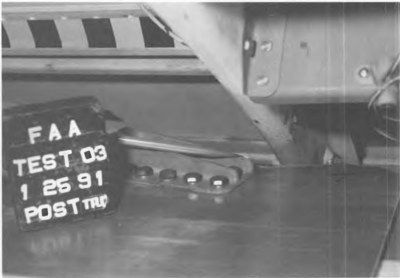
Figure 149. POST-TEST BIN 'B' 60" BIN DRAG LINK FITTING/FUSELAGE CONTACT, MARKS ON DRAG LINK FITTING
