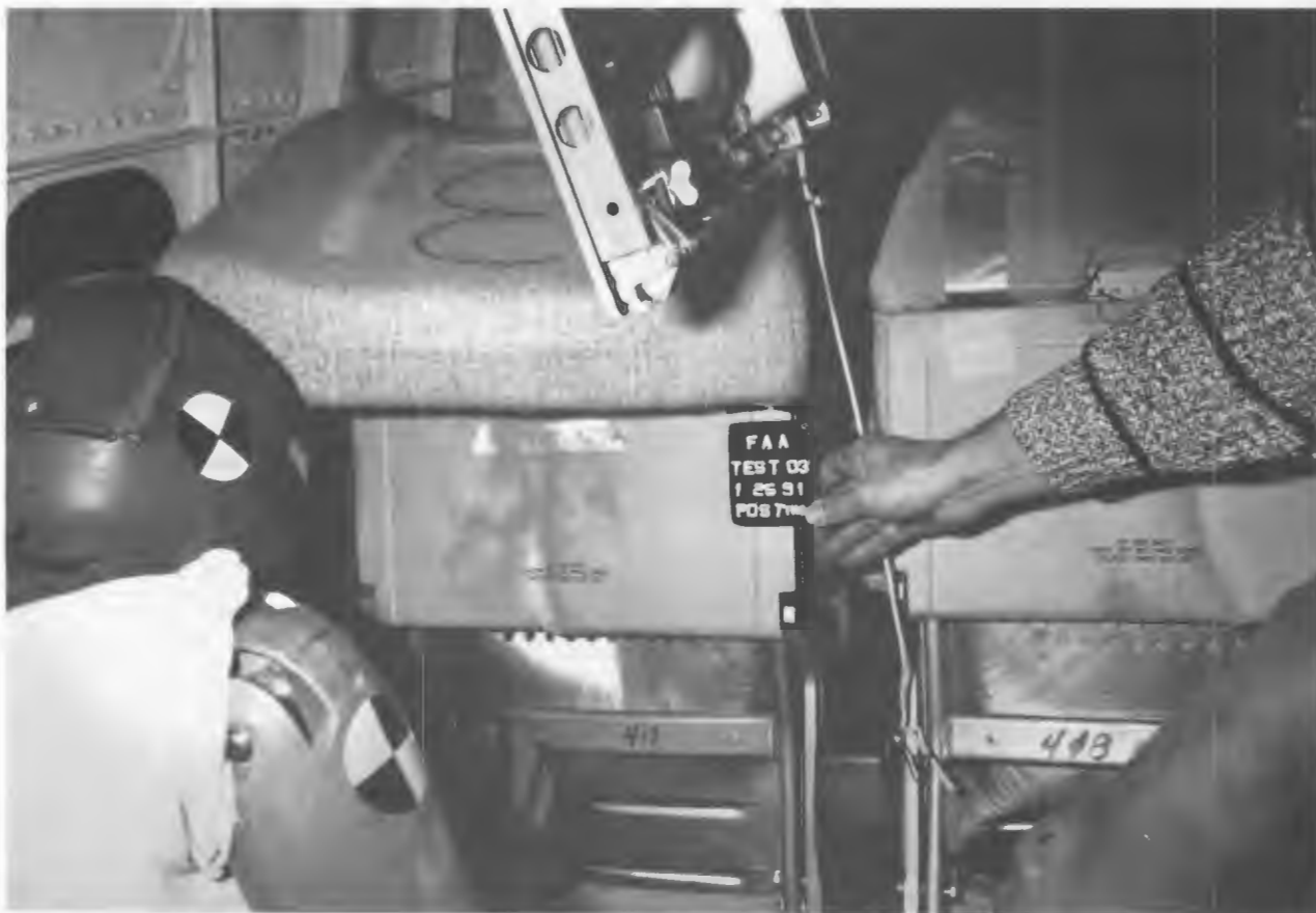
Figure 164. POST-TEST FRONT SEAT OUTBOARD SEATBACK REAR DUMMY CONTACT
