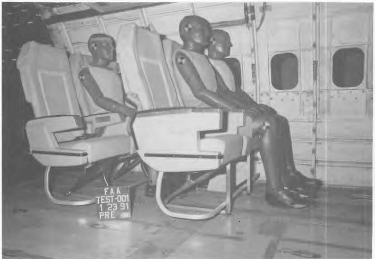
Figure 35. PRE-TEST SEATS AND DUMMIES FRONT ANGLE VIEW
