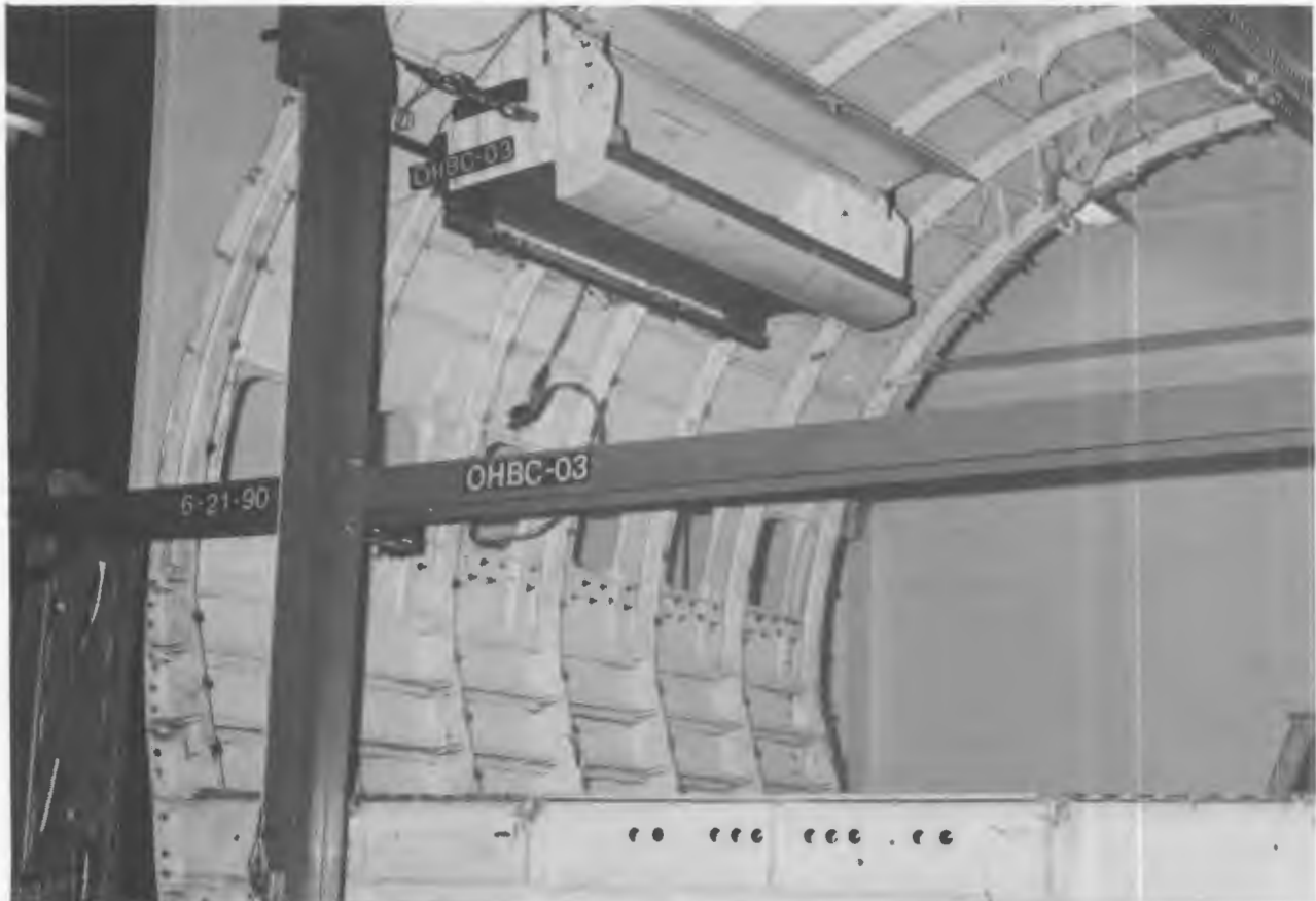
Figure C-25. ANGLE VIEW OF FUSELAGE AND STATIC TEST FIXTURE, TEST OHBC-03
