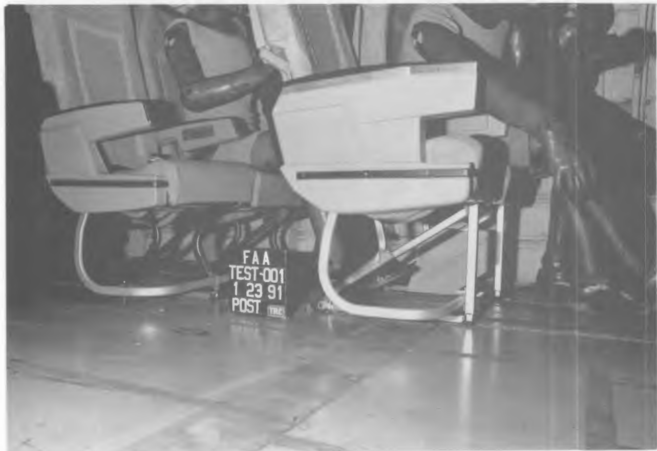
Figure 67. POST-TEST SEAT/FLOOR ATTACHMENTS
