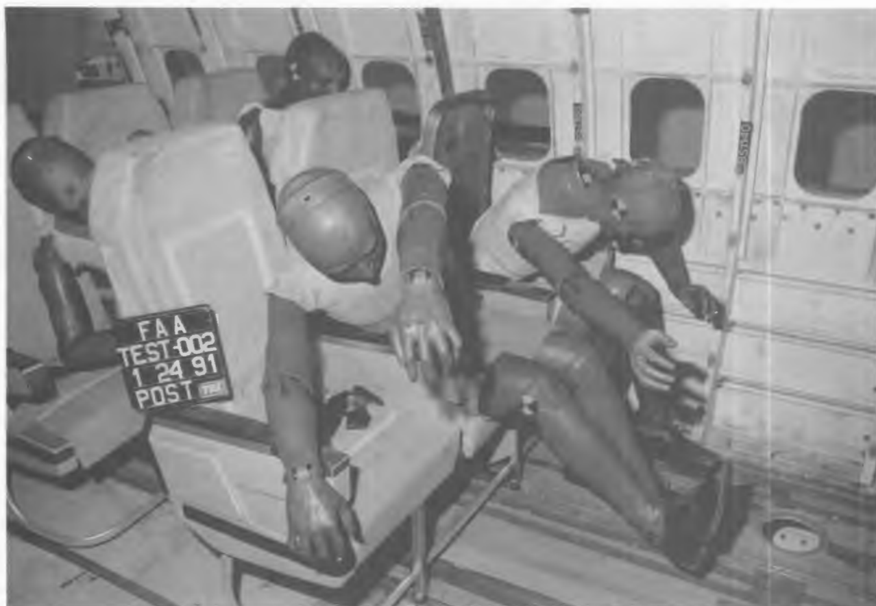
Figure 116. POST-TEST SEATS AND DUMMIES FRONT ANGLE VIEW
