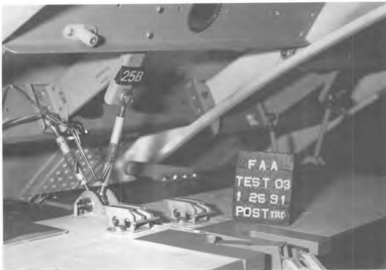
Figure 139. POST-TEST BIN 'B' LINKS 17 AND 25
