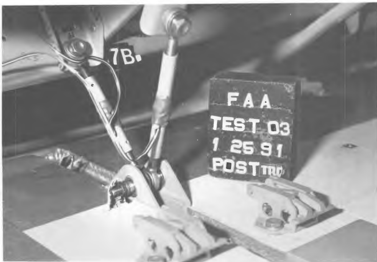
Figure 140. POST-TEST BIN 'B' LINKS 17 AND 25 REAR ANGLE CLOSE-UP
