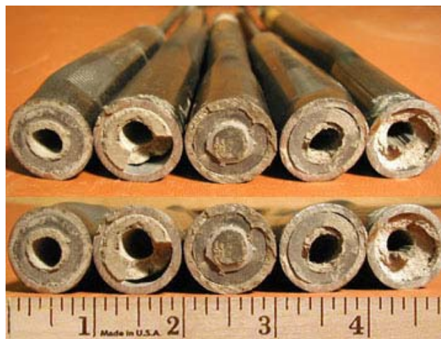
Figure 3.4 - Unconditioned CFRP Grip Failure
