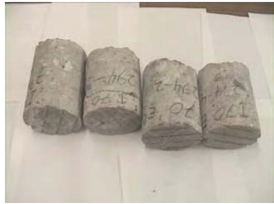
Fig. C.7.9 Concrete cores of 4 inch diameter
