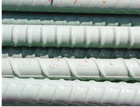
Fig. 2.3 A close view of the epoxy-coated rebars. Corrosion started on the locations with damaged coatings.
