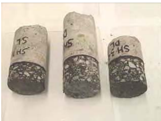
Fig. C.2.7 Concrete cores of 3 inch diameter
