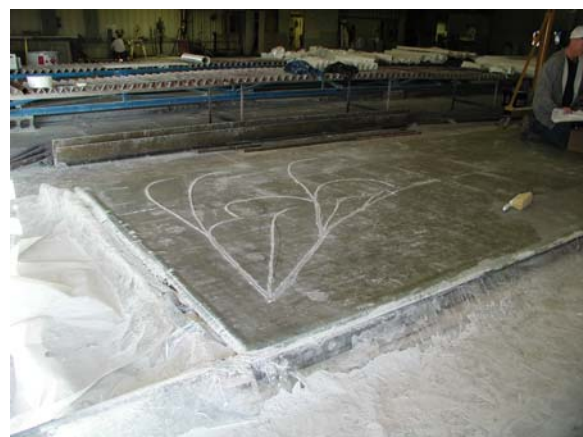
Fig. 3.8 Construction of GFRP panels (on the top surface are wires for embedded fiber optic sensors).
