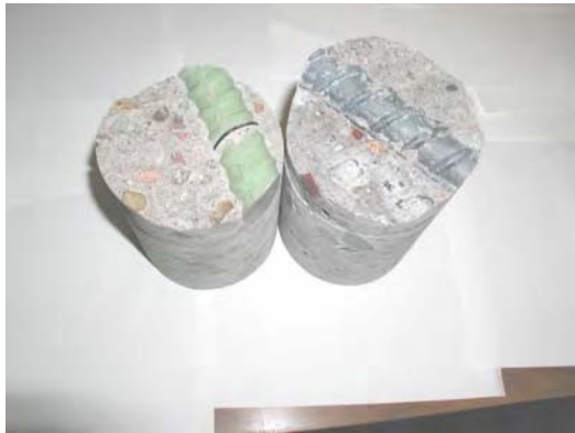
Fig. C.5.10 Core samples – from the south and north Bounds (ECR and black bar)
