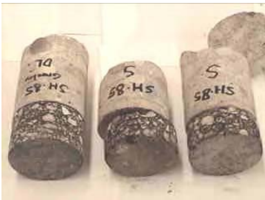
Fig. C.1.10 Concrete cores of 3 inch diameter
