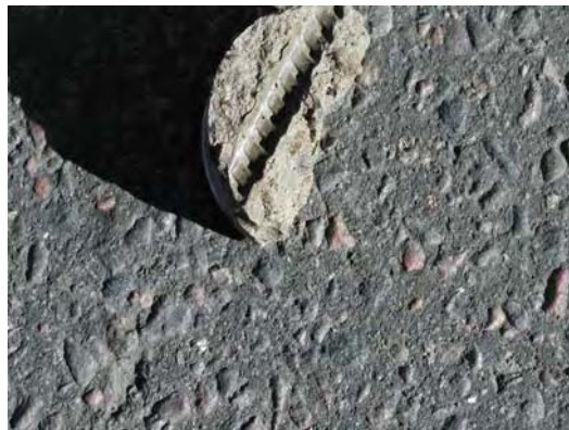
Fig. C.9.8 No signs of corrosion rust/deposit found on the concrete cover on an epoxy-coated rebar
