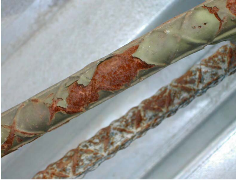
Fig. B1.1.3 Close view of corrosion of epoxy-coated rebars
