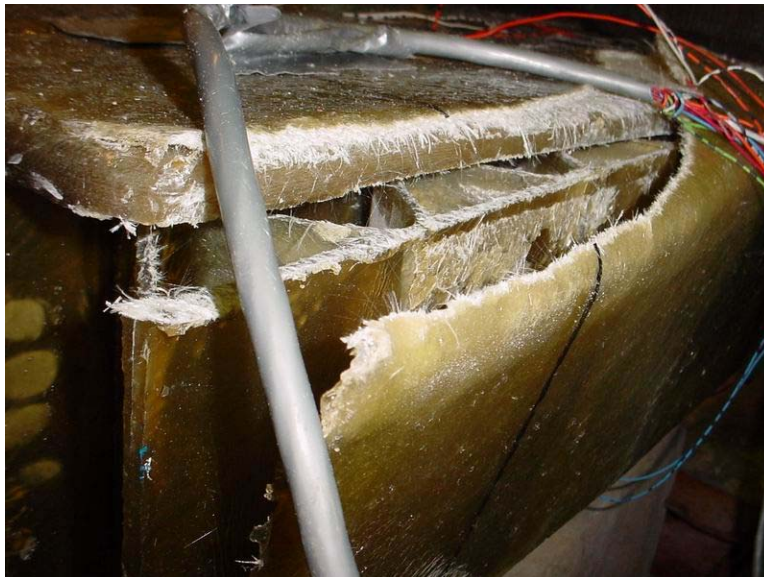
Figure 5-45 Debonding at the face-core interface in Test 4
