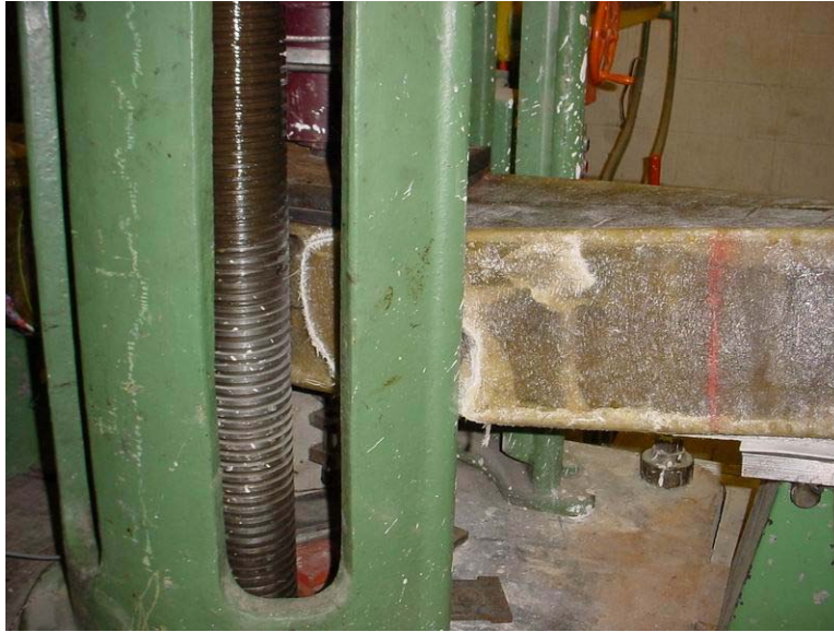
Figure 5-16 Failure mode in Test 1 – side view
