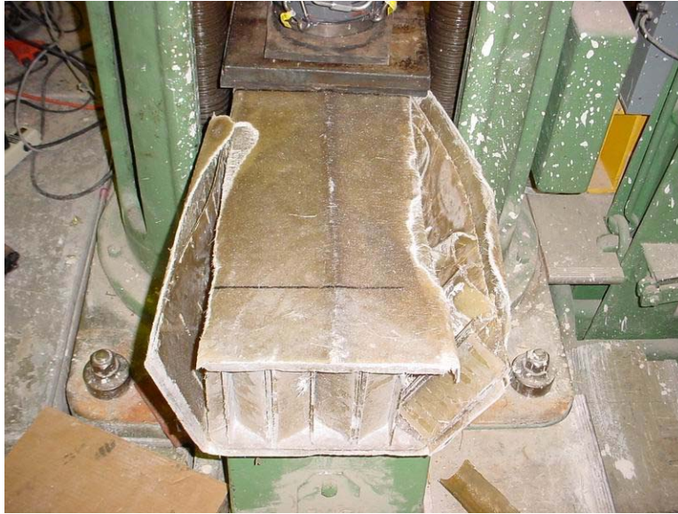
Figure 5-29 Buckling of the core in Test 2
