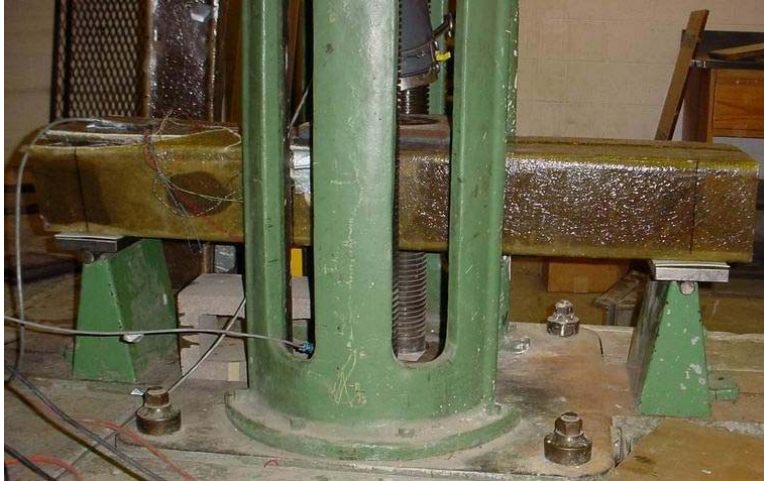
Figure 5-7 Beam test setup
