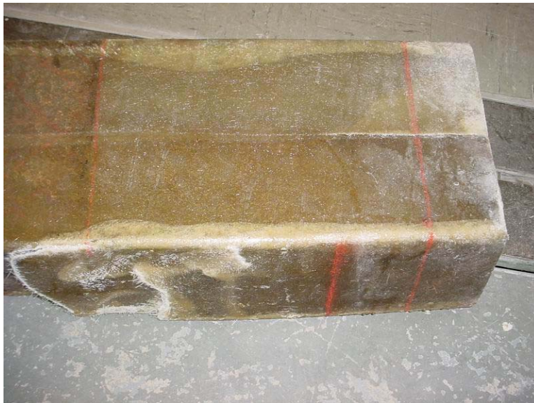
Figure 5-17 Local buckling of the core in Test 1
