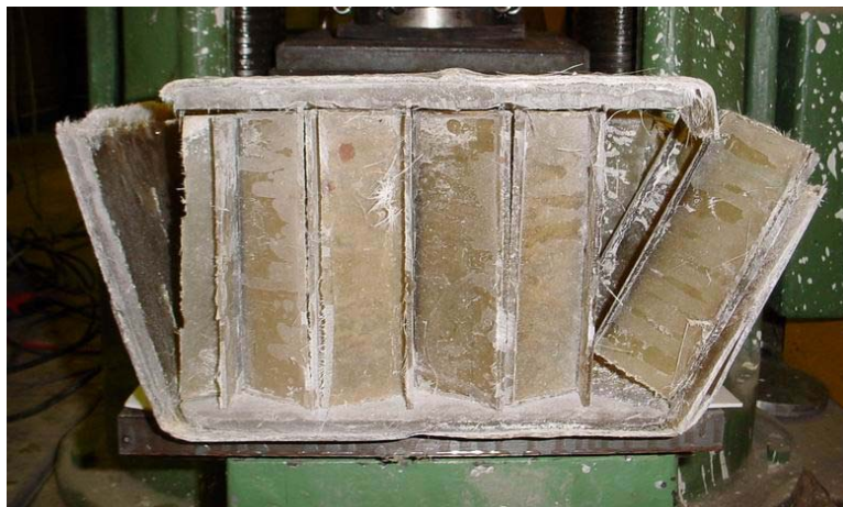
Figure 5-28 Debonding at top face-core interface in Test 2
