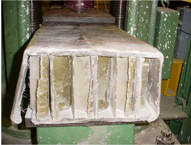
Figure 5-18 Failure mode in Test 1 – end view
