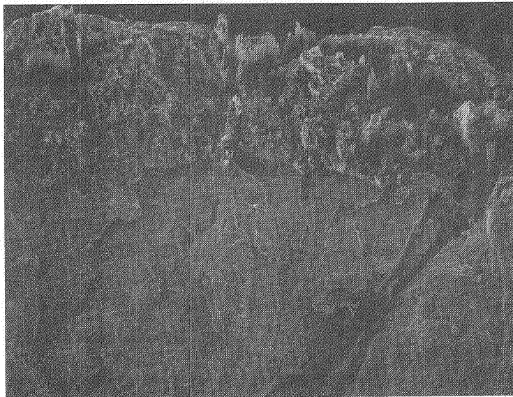
Secondary electron detector image of trans laminate flexure specimen. Note high degree of resolution but lacking contrast.
