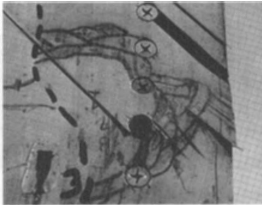
Figure 2-11. Rockwell Flaw Criticality Study Defect 12: Fiber Breakaway From Impact Surface
