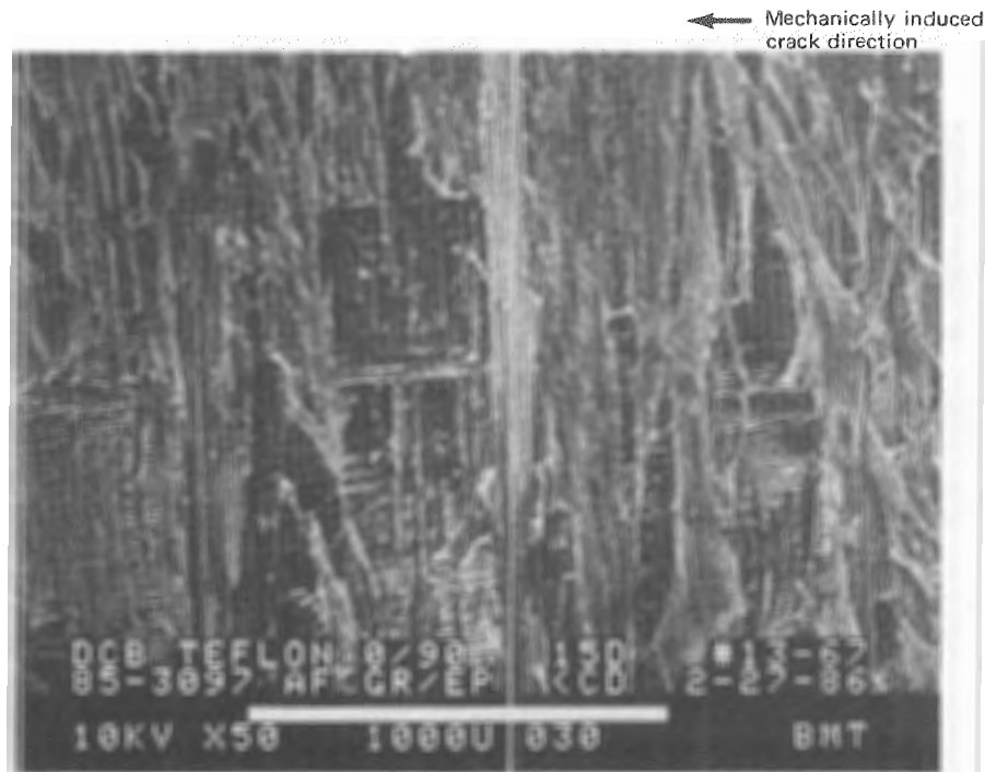
Figure 6-25. SEM Micrograph of a Teflon-Contaminated Tension Specimen
