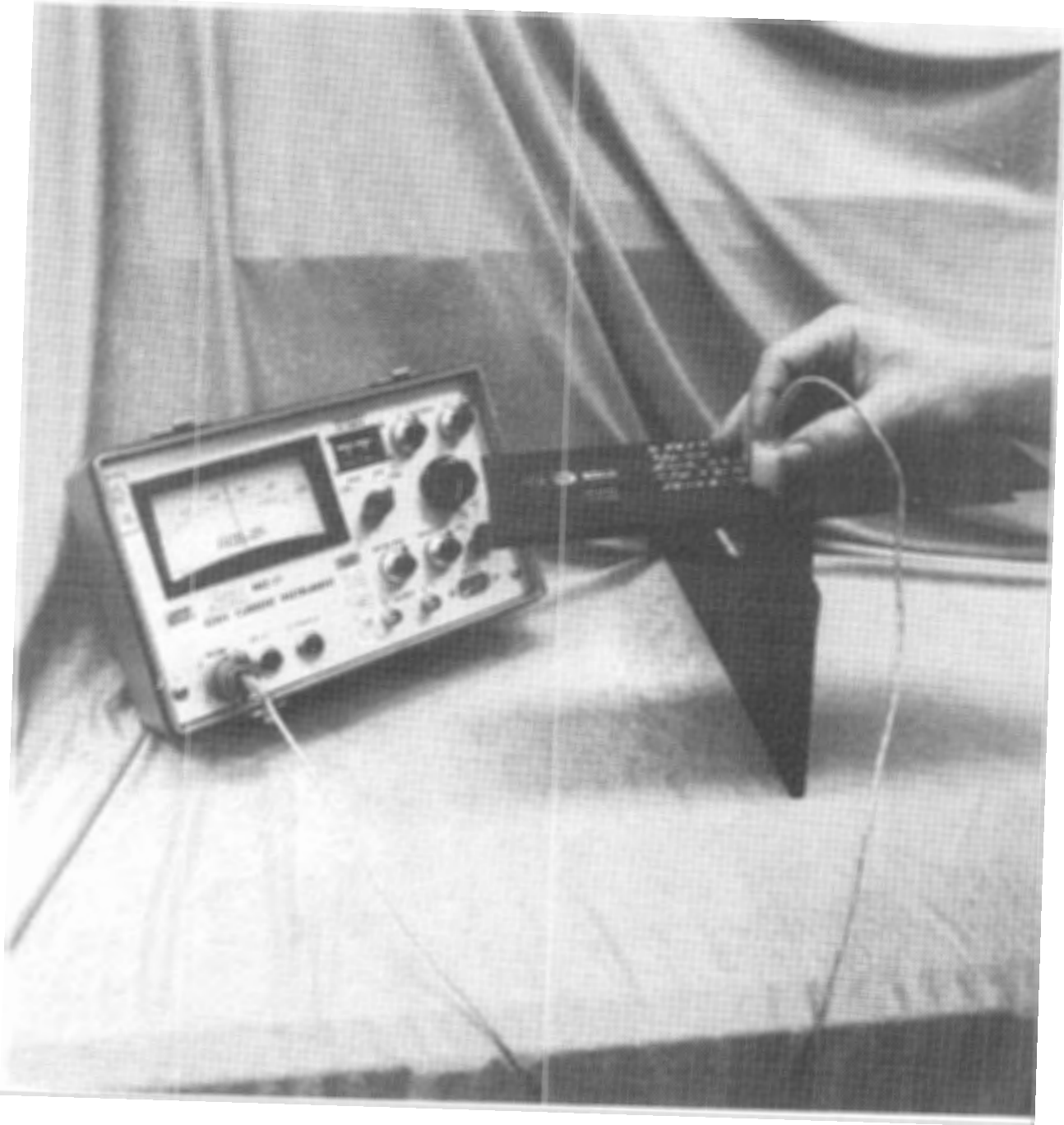
Figure 5-8. Typical Inspection Procedure Using Probe to Detect Subsurface Damage in Fabric Laminates
