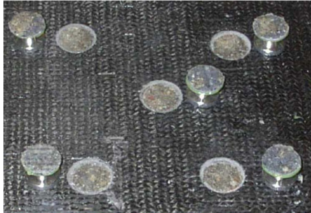
Figure 2-22 CFRP surface after a pull-off test
