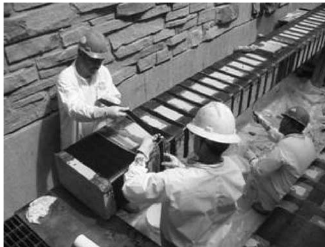
Figure 1-40 Placing final transverse wrap on AR specimen. The man below the beam is rolling more epoxy into the freshly applied wraps.
