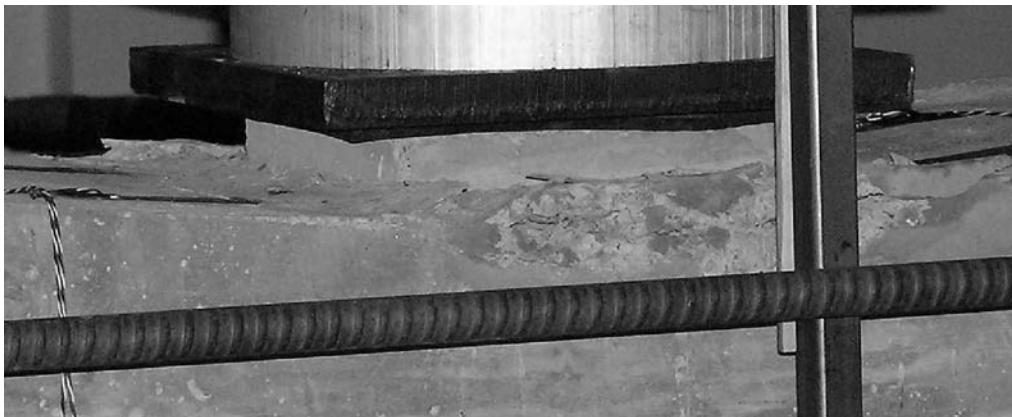
Figure 1-47 Concrete spalling around central cap (AC specimen)
