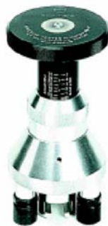
Figure 2-19 The pull-off test apparatus
