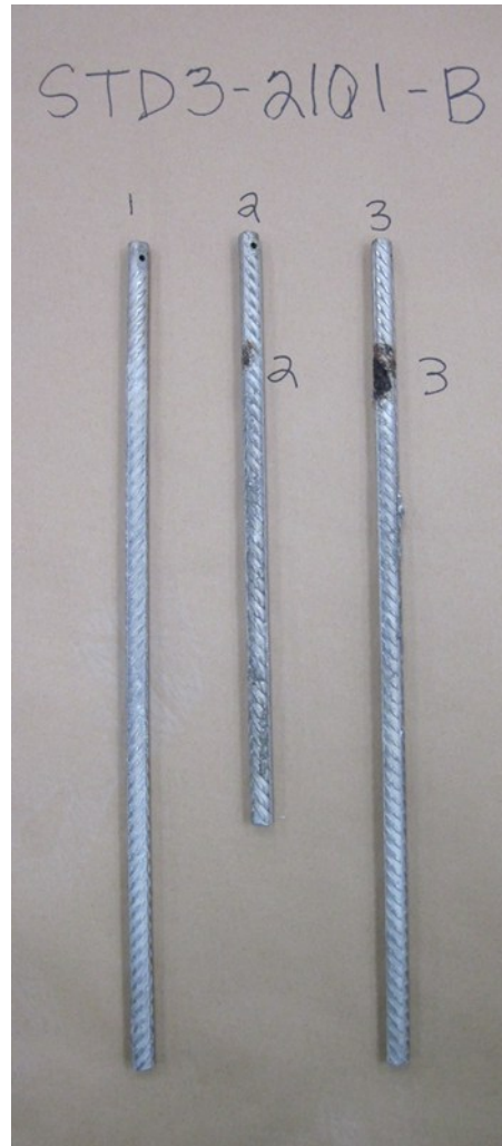
Figure 8-16. All rebars of sample STD3-2101-B.
