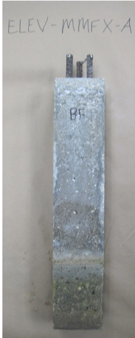
Figure 8-13. Back side of sample ELEV-MMFX-A before termination.
