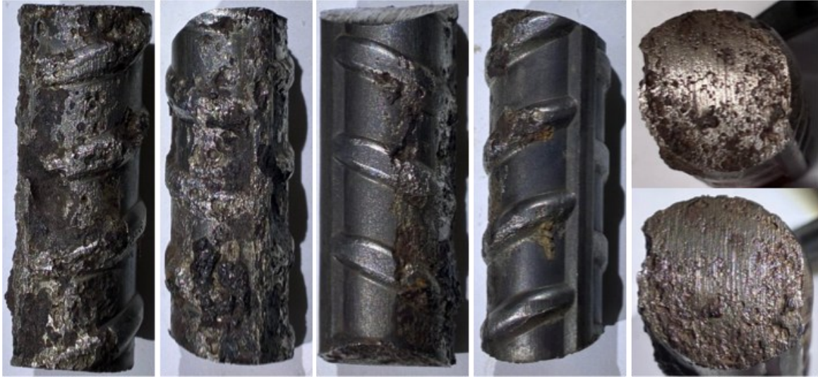
Figure 5-45. MMFX rebar section after additional immersion in cleaning solution.
