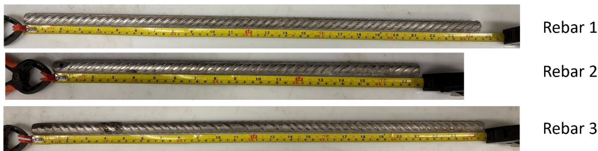
Figure 8-39. All rebars of sample STD3-2101-B after cleaning.
