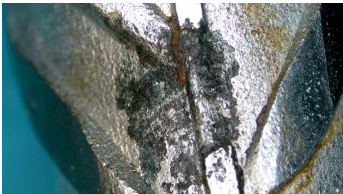
Figure 8-40. Corrosion spot observed on rebar 2 of STD3-2101-B.
