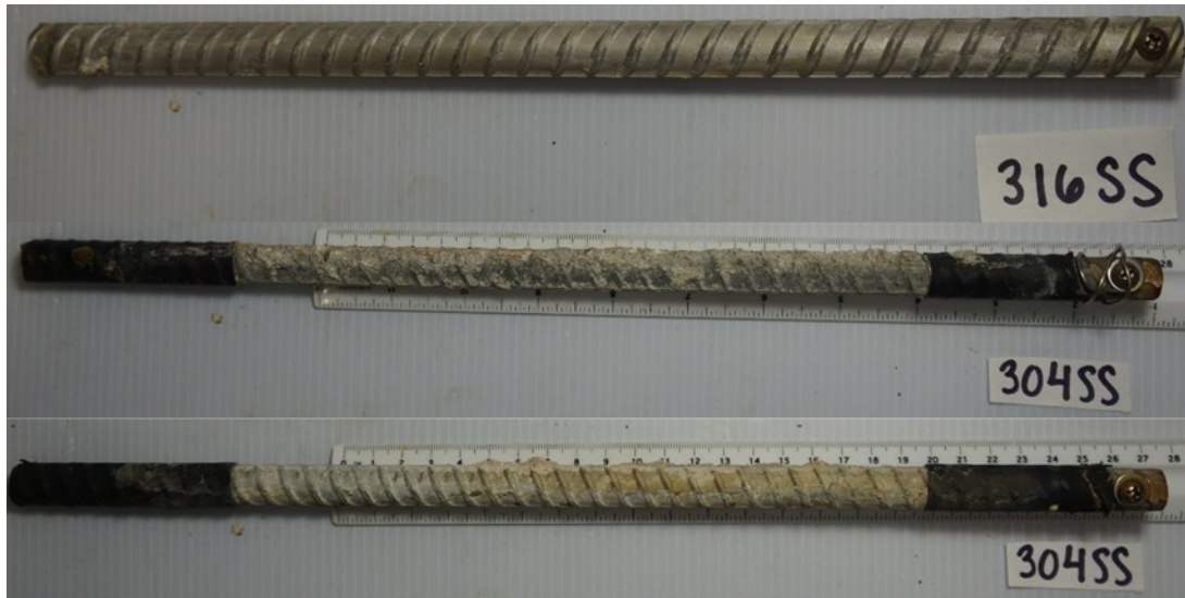
Figure 7-19. Images of one 316 SS rebar and two 304 SS rebars before cleaning.
