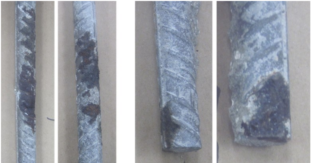
Figure 8-27. Corrosion spots on rebar 1 (right 2 images) and 2 (left) of sample STD3-3CR12-E.
