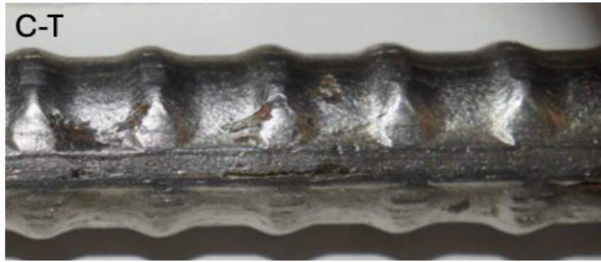
Figure 7-38. Closeup of pits on cladding, top face of 4-CCON-CT2-1 rebar C.
