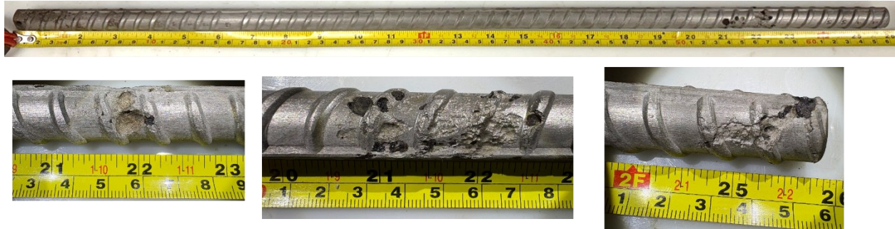
Figure 8-55. ELEV-MMFX-A - full length of rebar 3 and notable areas of corrosion damage.
