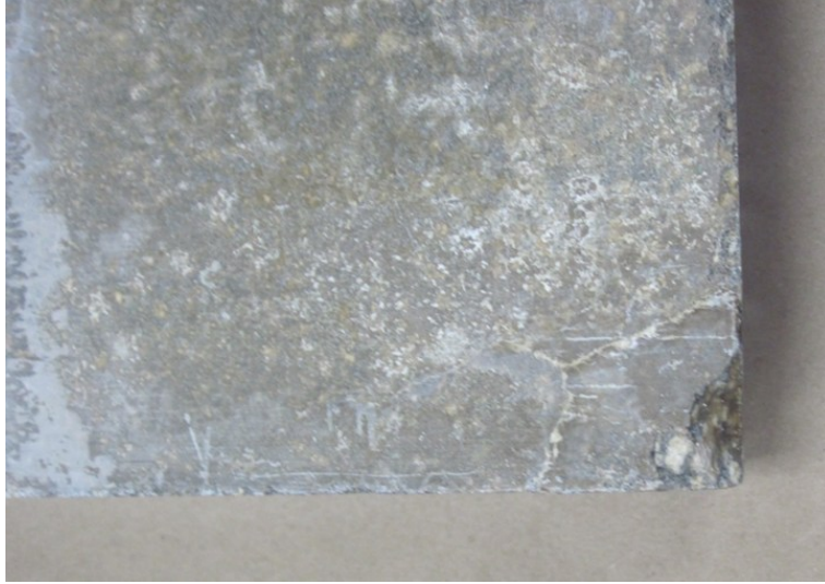
Figure 8-9. Back side crack of sample STD3-3CR12-E before termination.
