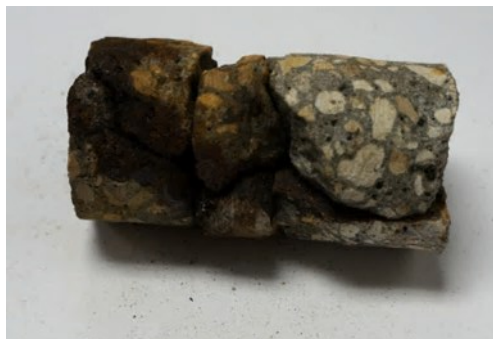
Figure 5-30. Image shows the core obtained from column 2101-A (~20 inches above WL).
