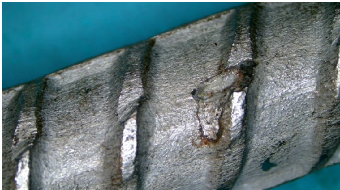
Figure 8-45. STD3-304-C (BENT) rebar 3 corroding site after cleaning.
