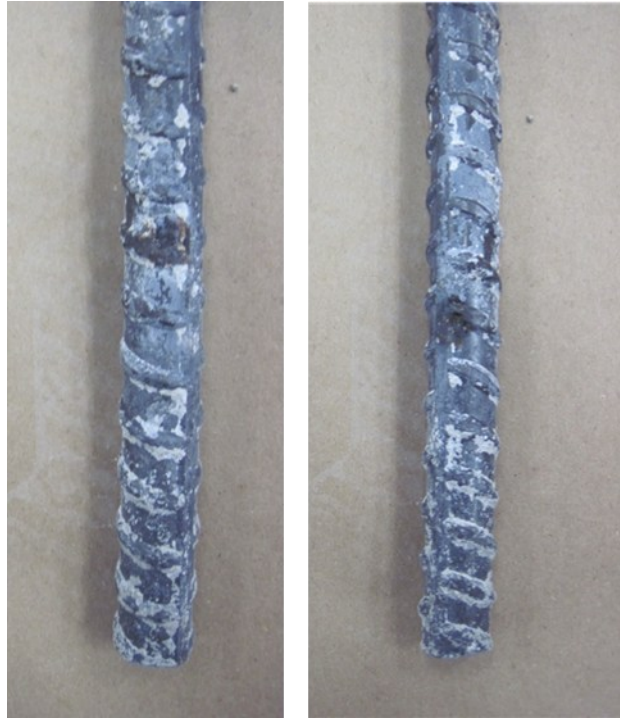
Figure 8-34. Corrosion spots on rebar 1 of sample ELEV-MMFX-A.
