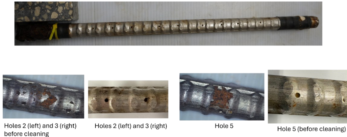
Figure 7-59. Top side of rebar C and select segments of sample CSDB-CT2-1.
