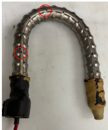
Figure 8-56. Rebar removed from UBDB-SMI-B sample: left top side full U rebar view and two close-up of the drilled holes.
