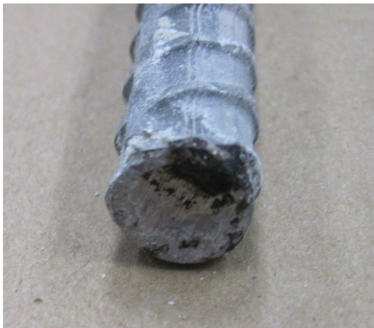
Figure 8-23. Close up corrosion spot on end of rebar 2 of sample BENT-STD3-304-C.
