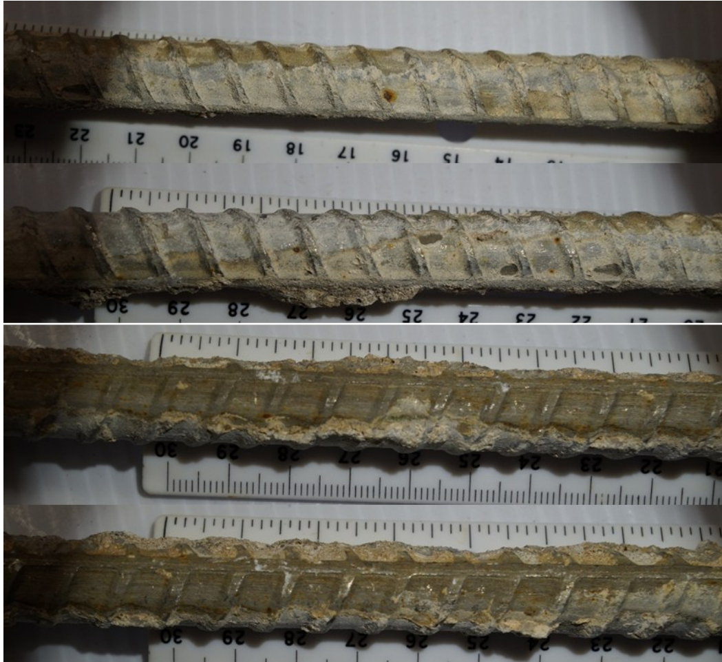
Figure 7-22. Closeups of pitting corrosion on 304SS rebars.
