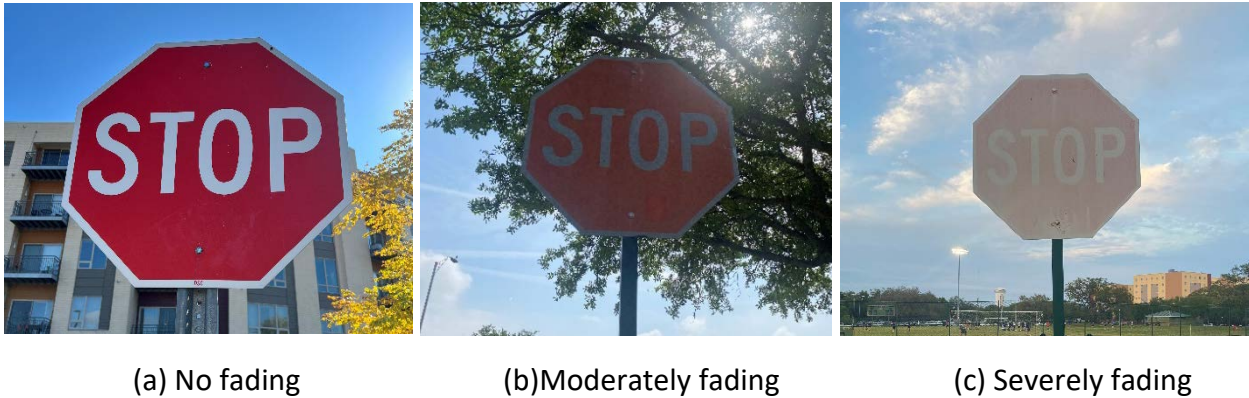
Figure 3-14 Example of a fading stop sign.
