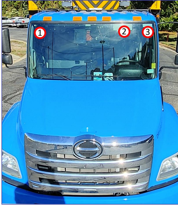
Figure 18. RCTMA Three Front-Facing Camera Locations
