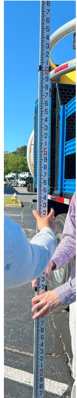
Figure 43. Level Rod used for visibility test
