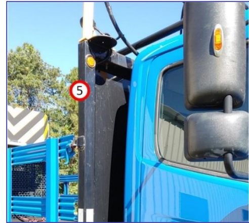
Figure 19. RCTMA Rear-Facing Camera Locations
