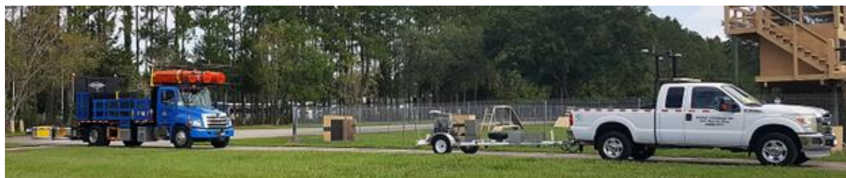
Figure 1. ATMA system as used in the proof-of-concept project BDV 31-977-133. The autonomous follower vehicle (blue) is shown on the left with a crash attenuator deployed at the back (yellow). The white vehicle on the right is an FDOT truck retrofitted with the necessary equipment to act as a leader vehicle.
