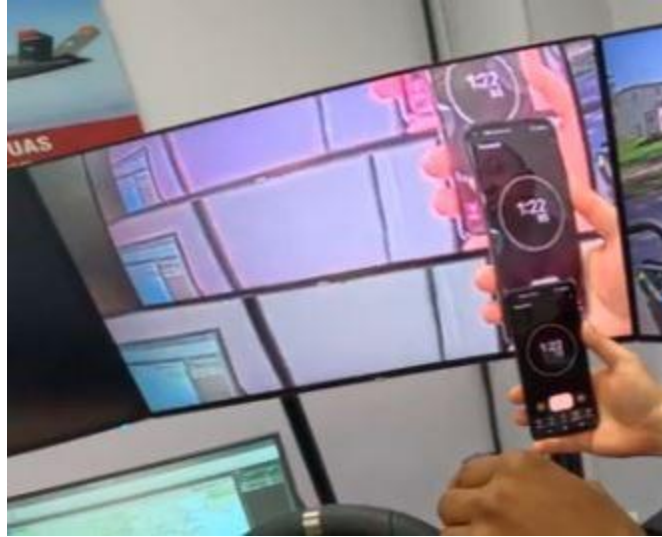
Figure 33. Latency Test 1, showing multiple images in the C2 monitor used for comparison of stopwatch times
