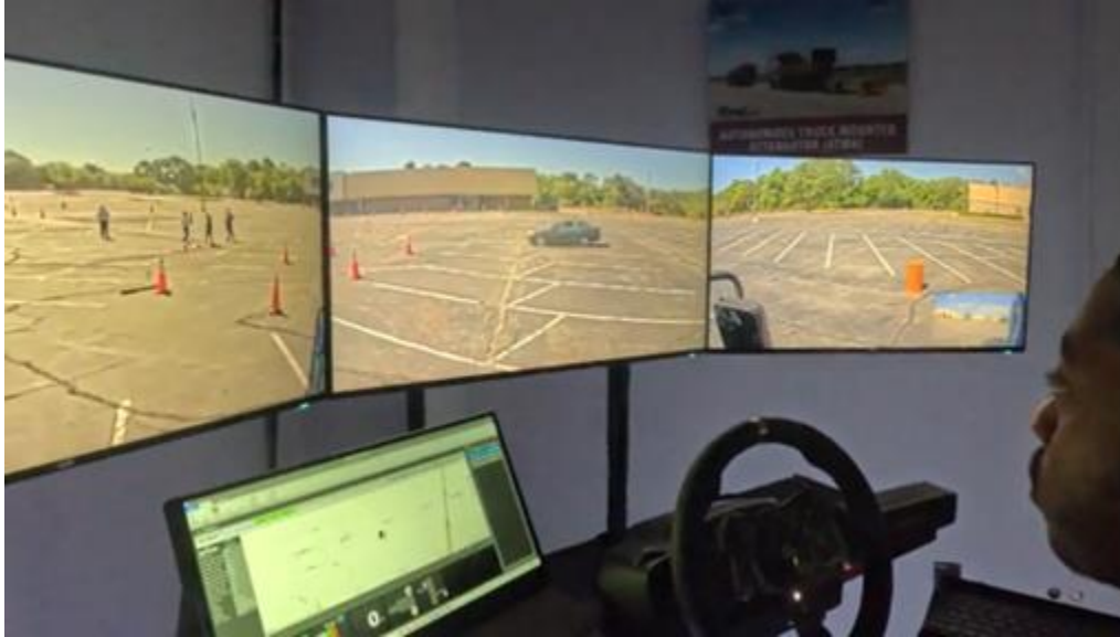
Figure 40. Monitor view during obstacle detection and braking test
