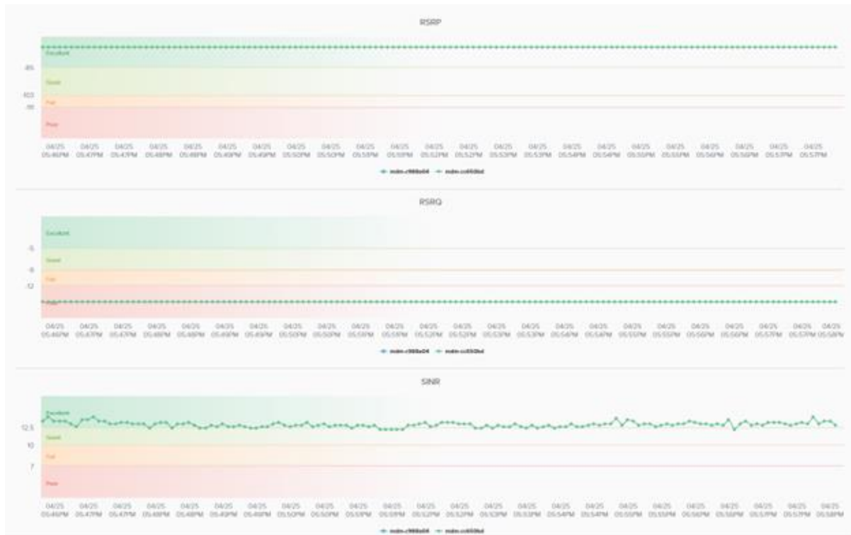
Figure 31. Graphs showing signal parameters RSRP, RSRQ, and SINR for the C2-RCTMA connection. This data is representative; they were not available from the April 15 testing session.
