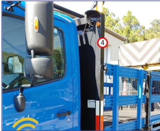
Figure 19. RCTMA Rear-Facing Camera Locations
