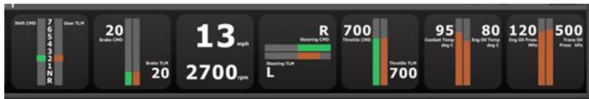
Figure 26. The C2 driver is provided with readouts for the RCTMA's functions on the laptop shown in Figure 10. From left to right, the readouts are gear, brakes, mph and rpm, steering, throttle, coolant and engine oil temperatures, engine oil and transmission oil
