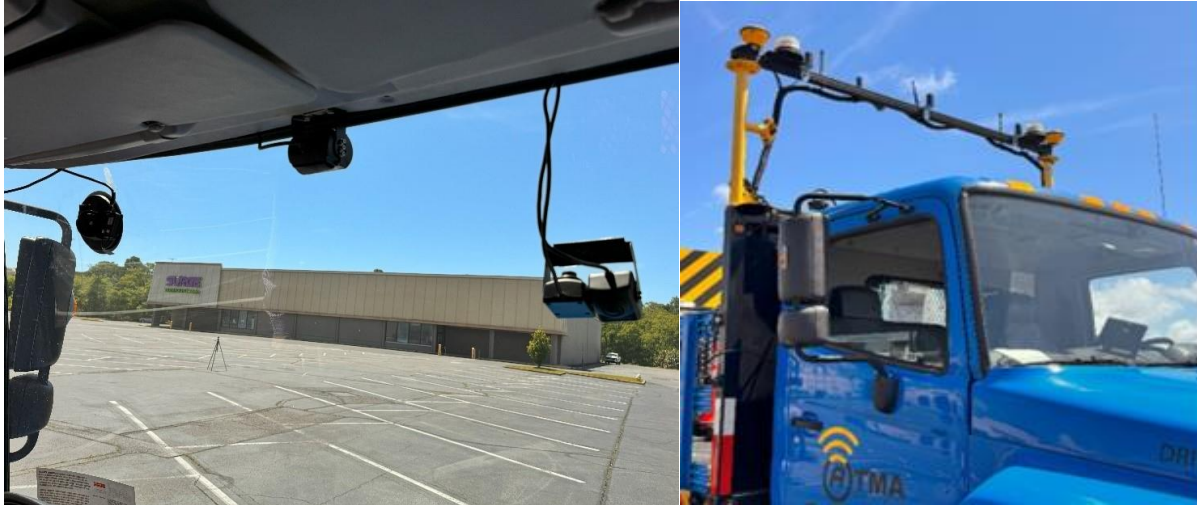
e) The camera placement inside and above the RCTMA
