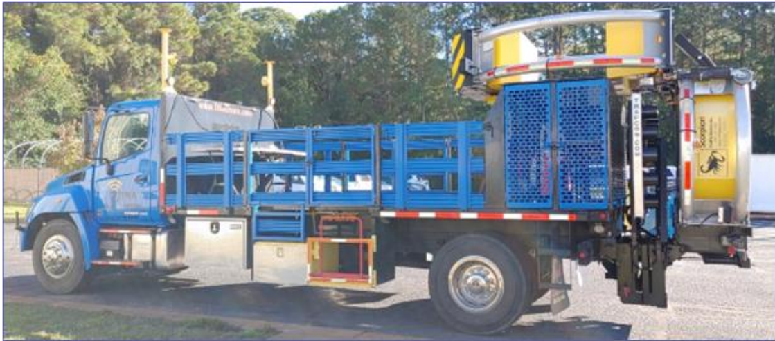
Figure 4. Kratos autonomous truck-mounted attenuator (ATMA)
