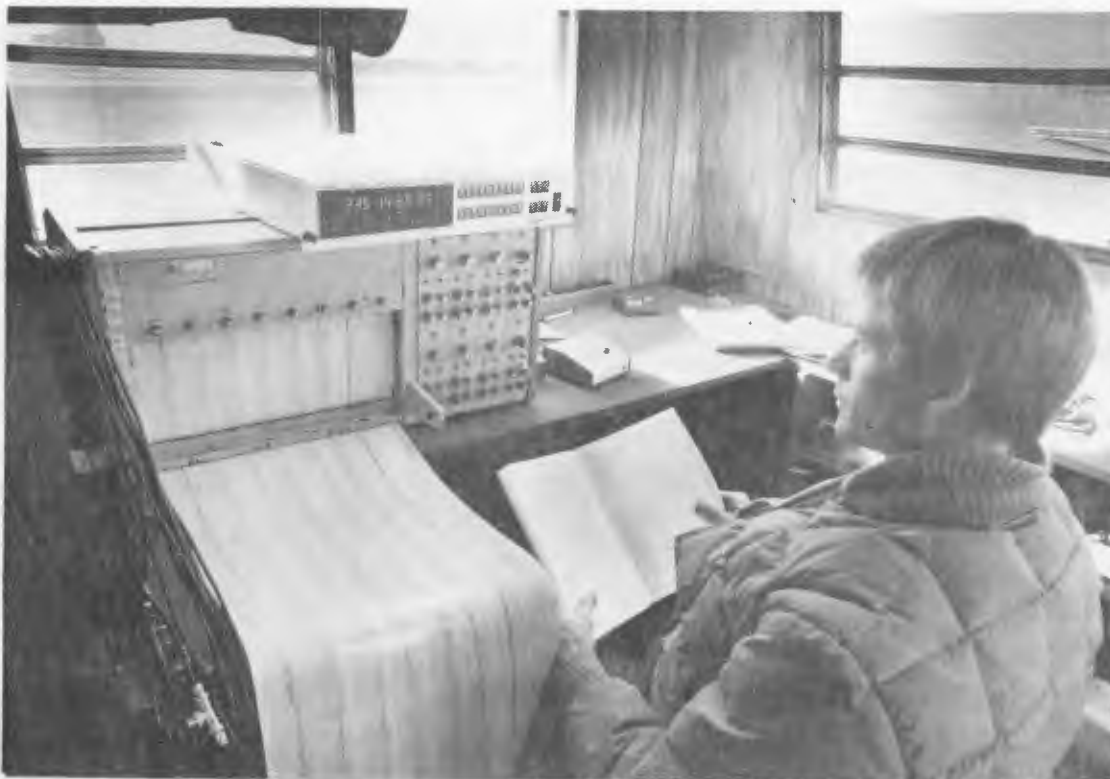
FIGURE 31. MOBILE LABORATORY EQUIPMENT -- AN 8-CHANNEL STRIP CHART RECORDER, TIME CODE GENERATOR, AND EVENT MARKER
