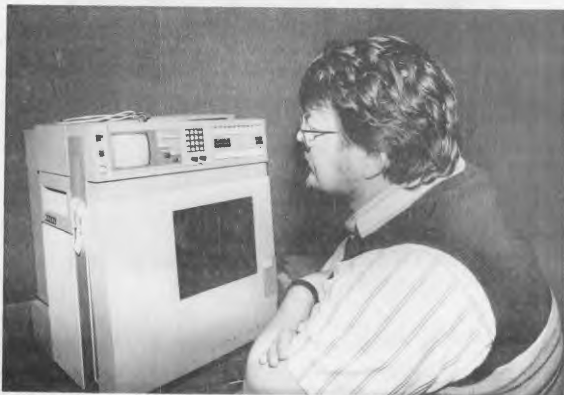
FIGURE 32. A 14-CHANNEL RACAL MAGNETIC TAPE RECORDER USED TO STORE TEST EQUIPMENT SIGNALS
