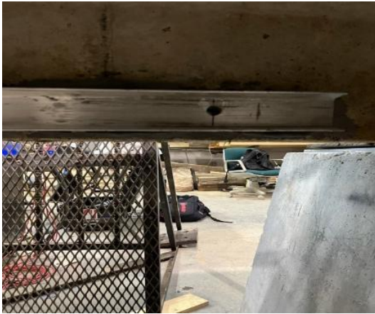
b) End bolt rupture for Specimen SEB.
