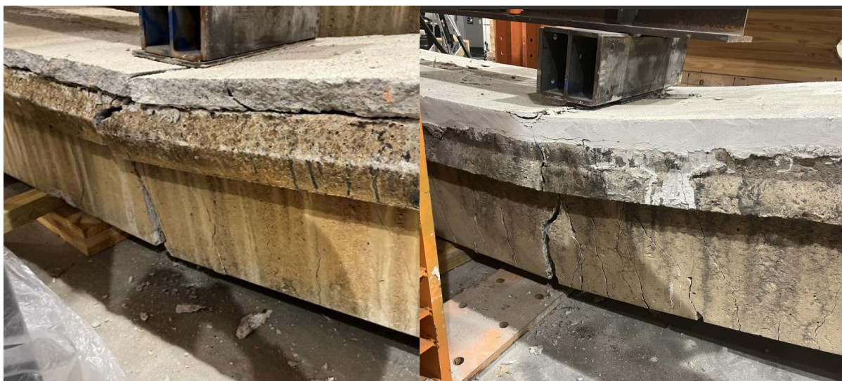
Figure 0.4 Failure of specimen L2 (left); and L3 (right).
