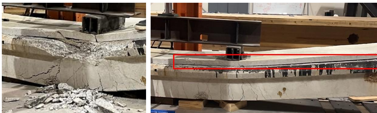
Figure 7.5 Flexural failure of L4 (left); and topping delamination before failure (right).
