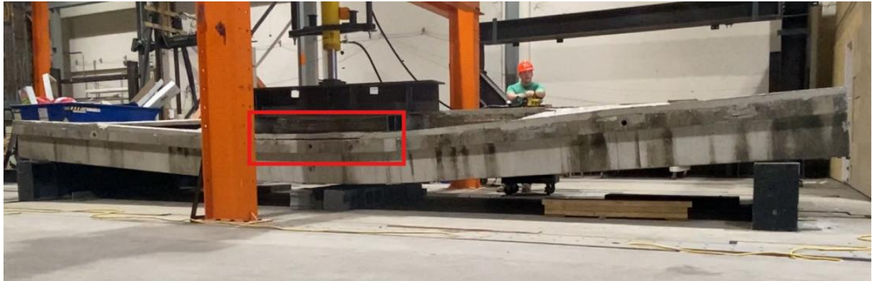
Figure 0.2 Delamination of LMC on girder L1.
