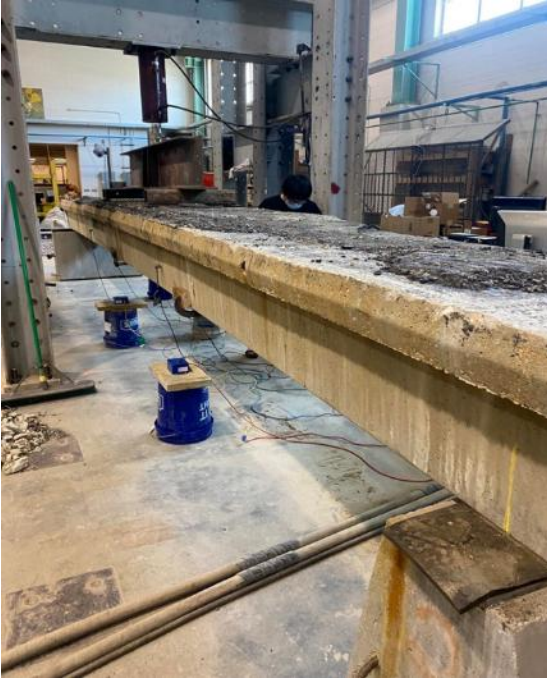
Figure 3.3 Skinny leg channel girder test setup; (left) University of South Carolina, (right) Clemson University.
