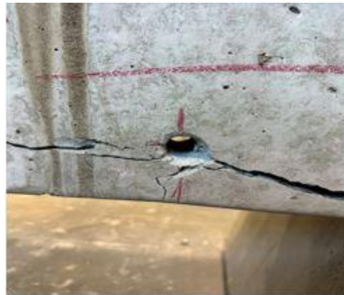
c) Concrete splitting at end bolt for Specimen SB.
