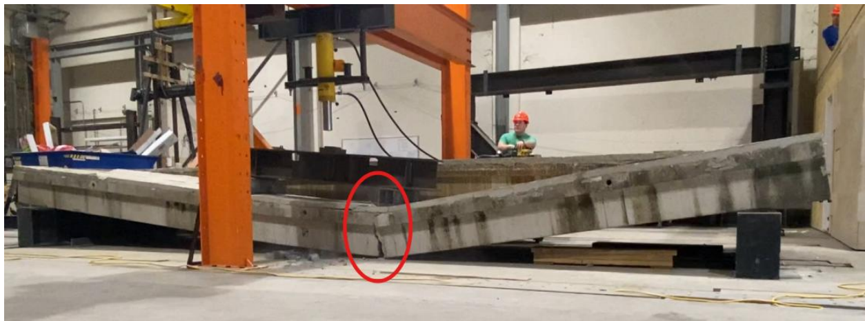
Figure 0.3 Failure of girder L1 due to strand rupture below load point.
