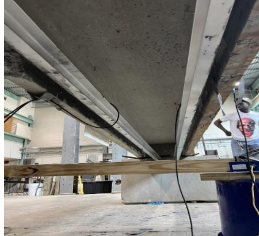
a) Debonding of the AA channels for specimen SE.
