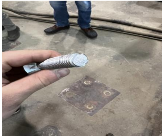
b) End bolt rupture for Specimen SEB.
