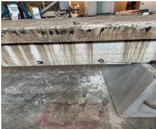
c) Concrete splitting at end bolt for Specimen SB.
