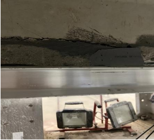
a) Debonding of the AA channels for specimen SE.
