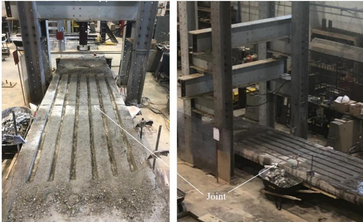
Figure 9.2 Lab specimen with near-surface mounted (NSM) bars.
