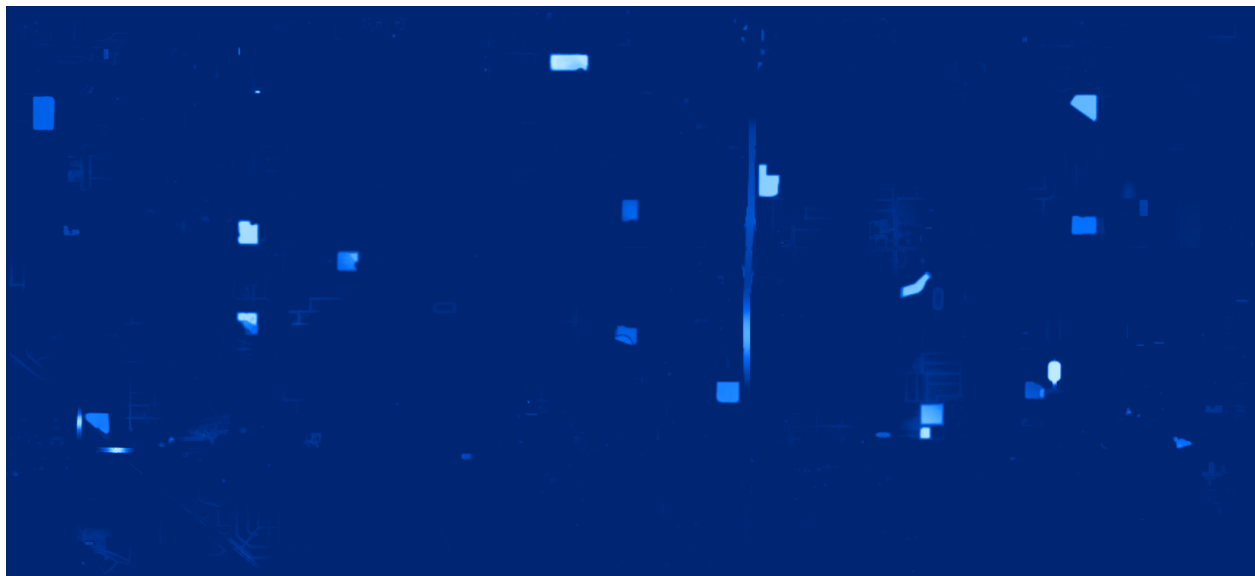
Figure 6. Example of Depression Depth Raster Derived from the Difference Between Filled and Original DEM Surfaces
