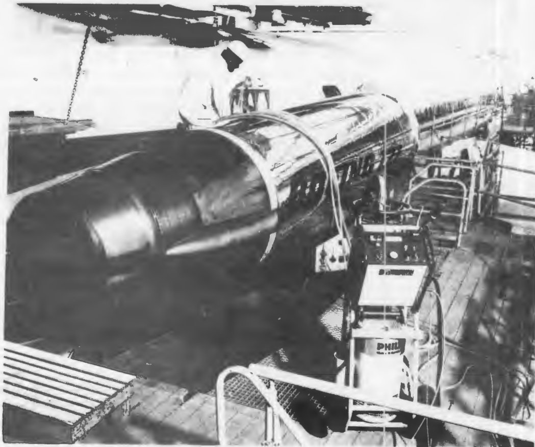
FIGURE 10. INSPECTING ENGINE MOUNT COMPONENTS FOR A BOEING 727 USING A MOBILE 160 kV X-RAY SYSTEM Courtesy of Philips GmbH
