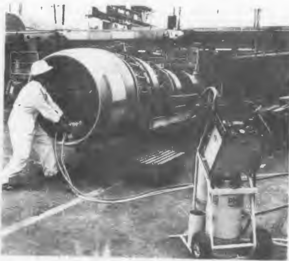
FIGURE 8. ENGINE INSPECTION USING A 160 kV METAL-CERAMIC X-RAY UNIT Courtesy of Philips GmbH
