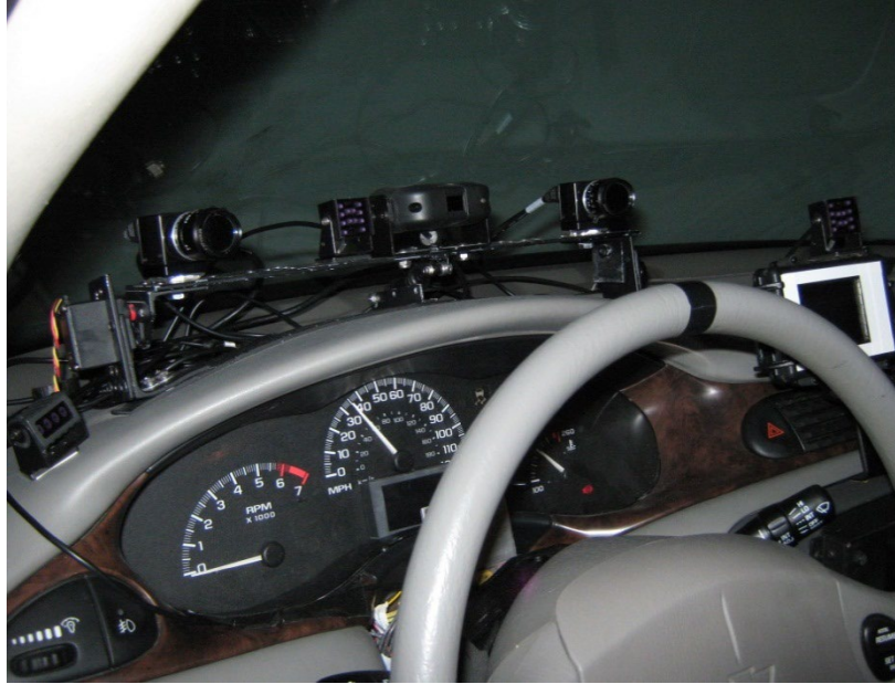
Figure 11. FaceLab cameras mounted in the Malibu cab with a separate head tracking system mounted between them
