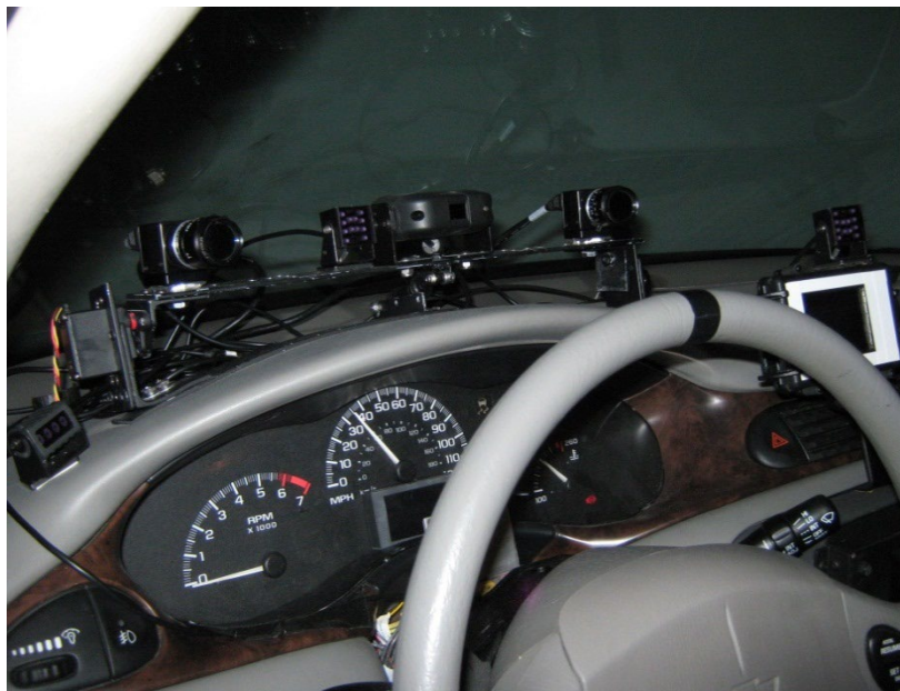
Figure A-1. FaceLab cameras mounted in the Malibu cab with a separate head tracking system mounted between them
